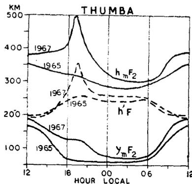
Figure 1. Daily variation of the height of the maximum ionisation ( $h_m F_2$ ), minimum virtual height ( $h'F$ ) and the semi-thickness ( $y_m F_2$ ) of the  $F_2$  layer at the equatorial station Thumba during the years 1965 and 1967.
