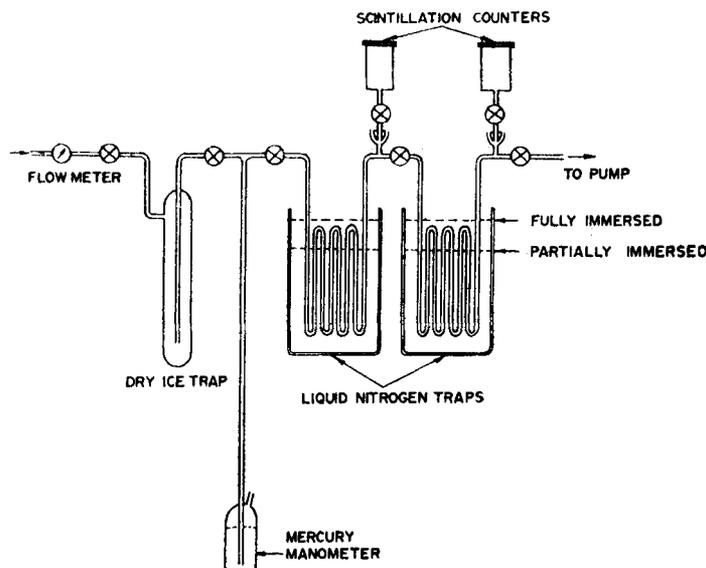
FIG. 1. Glass system used in the estimation of radon.
