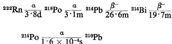
Fig. 1. Decay chain of  ${}^{222}\text{Rn}$
