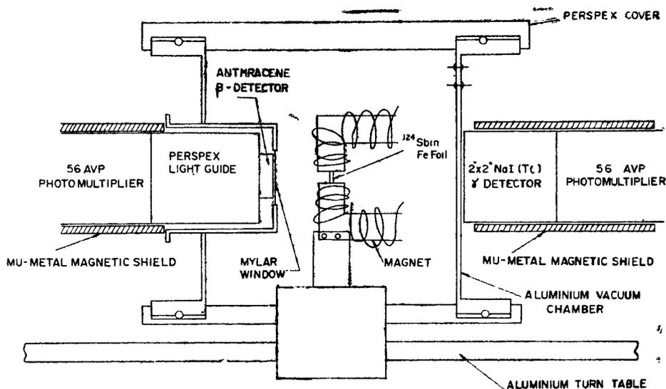
FIG. 3. Vacuum chamber assembly used for the  $\beta$ - $\gamma$  angular correlation studies showing the C type electromagnet used for the field measurements.
