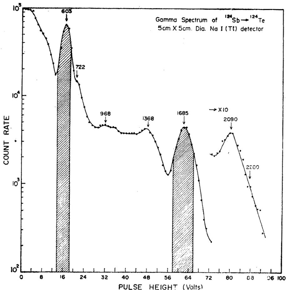
FIG. 2. Pulse height spectrum of  $^{124}\text{Sb}$  in Fe sample with 5 cm  $\times$  5 cm dia. NaI (Tl) detector. The gamma-ray energies are in keV. The single channel window settings used for  $\gamma$ - $\gamma$  angular correlation of 603-1685 keV cascade are shown as cross-hatched areas.
