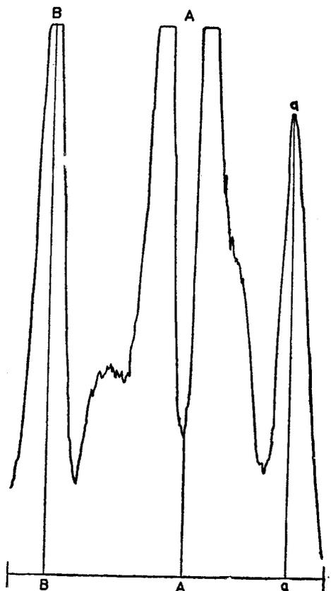
FIG. 3. 5027 Å lines of uranium, emitted by a microwave excited uranium iodide lamp operating at high temperatures, recorded on a Fabry-Perot spectrometer.
