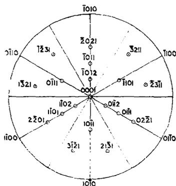
FIG. 3. Stereographic projection of anhydrous lithium nitrate.
