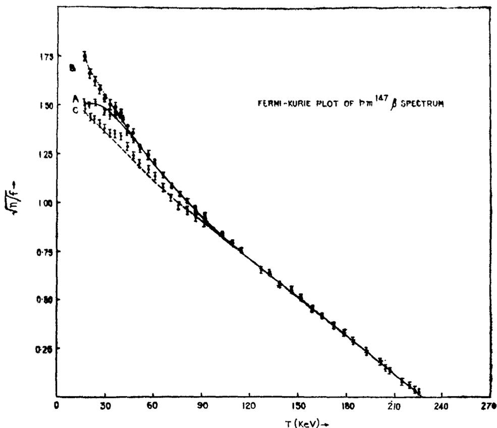
FIG. 2. Kurie plots of  $\text{Pm}^{147}$   $\beta$ -spectrum; A, uncorrected; B, corrected for window absorption; C, corrected for backscattering also.
