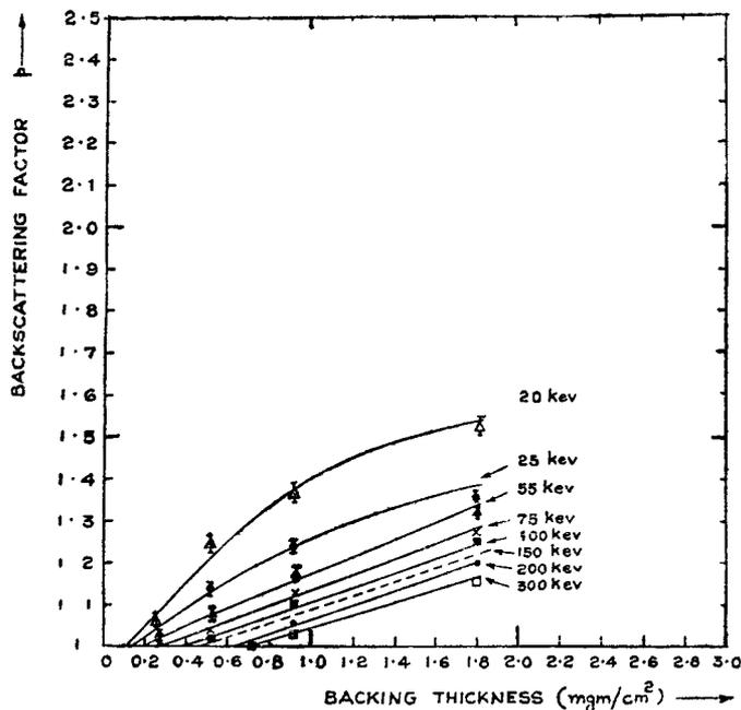
Fig. 1. Backscattering of low energy electrons in thin aluminium.
