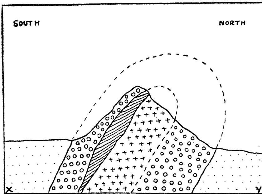
TEXT-FIG. 2. An Approximate Structural Section (along XY in the Map) showing an Isoclinal Fold
