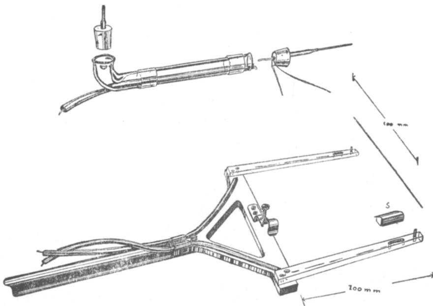
FIG. 3. Exploded diagram of the thermocouple psychrometer (S=aluminium shield)
