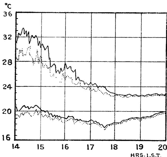
FIG. 5. "Dry" temperatures (upper two curves) and "wet" temperatures (lower two curves) at 10 cm. (straight lines) and 60 cm. (broken lines) above bare soil
