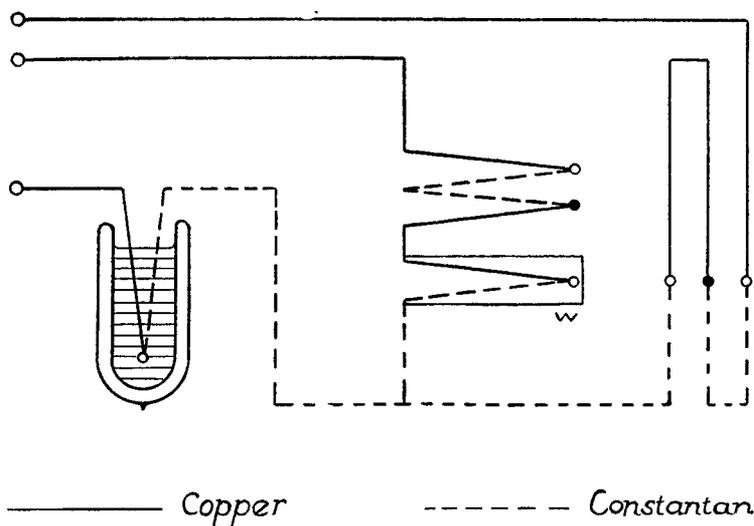
FIG. 4. Circuit of the thermocouple psychrometer compensated for the radiation error
