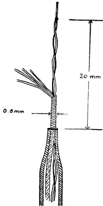
FIG. 2. Construction of the "Wet" needle, black: copper, white: constantan.
