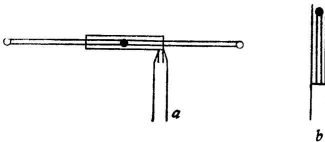
FIG. 1. "Wet" thermocouple, a: "L" type, b: needle type.
