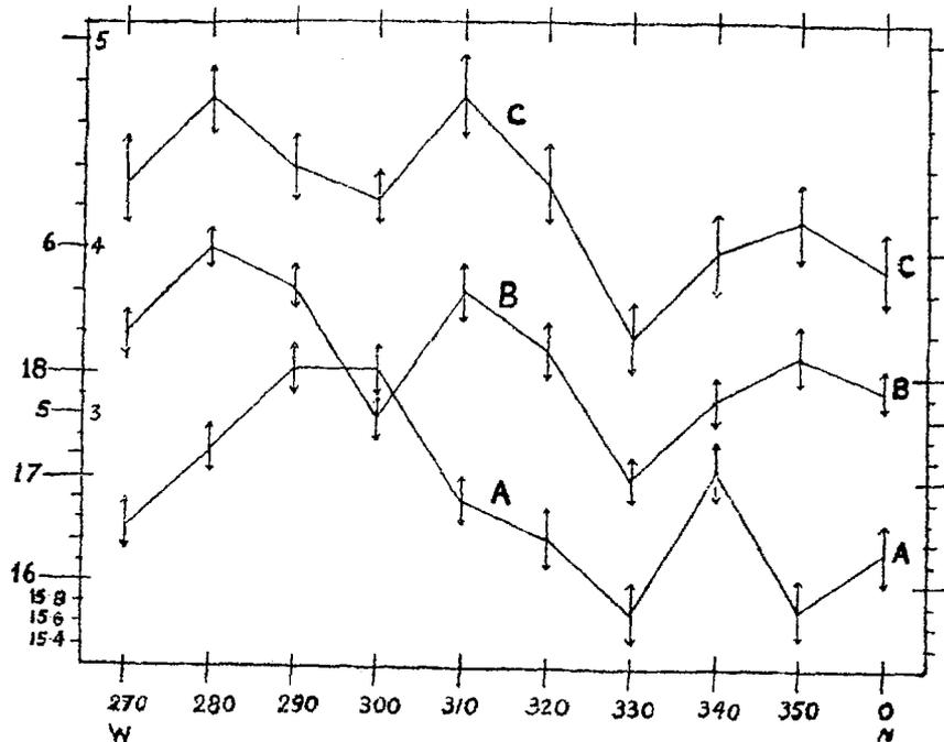
FIG. 1. The azimuthal variations of cosmic-ray intensity for a fixed zenith angle of  $60^\circ$  at Lahore. The vertical scale for each curve is given at the left.
