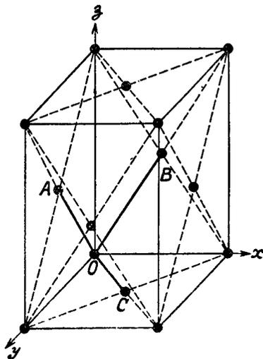
FIG. 4. Face-centred Orthorhombic Lattice
