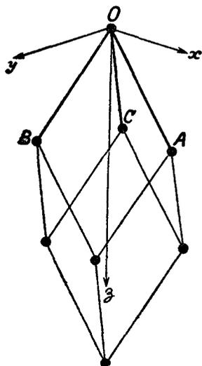
FIG. 5. Unit cell of the Rhombohedral Lattice
