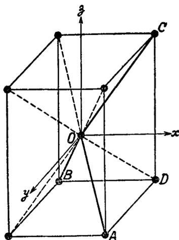
FIG. 3. Body-centred Orthorhombic Lattice
