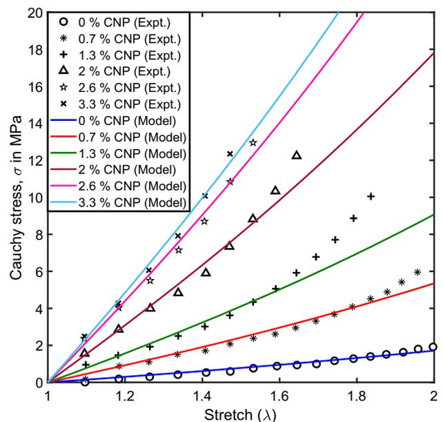
**Figure 3.** Validation of the model (8) with Mahmoud et al. experimental data [38] for a nitrile butadiene rubber (NBR) filled with different levels of carbon nanoparticles (CNPs).
