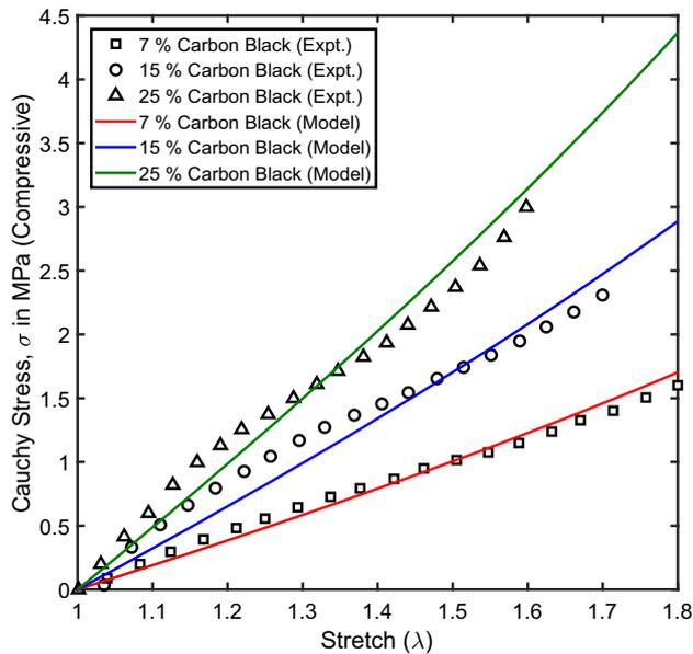
**Figure 2.** Validation of the model (8) with Bergstrom and Boyce experimental data [36] for a chloroprene rubber filled with different levels of N600 carbon black.
