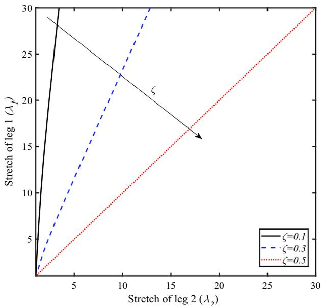
**Figure 5.** Relationship between stretch in legs 1 and 2 at different cut positions  $\zeta$ .
