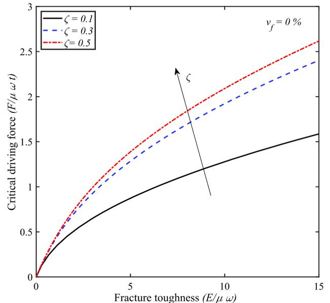
**Figure 6.** Critical driving force versus fracture toughness at different cut positions  $\zeta$  for an unfilled rubber elastomer ( $v_f = 0\%$ ).
