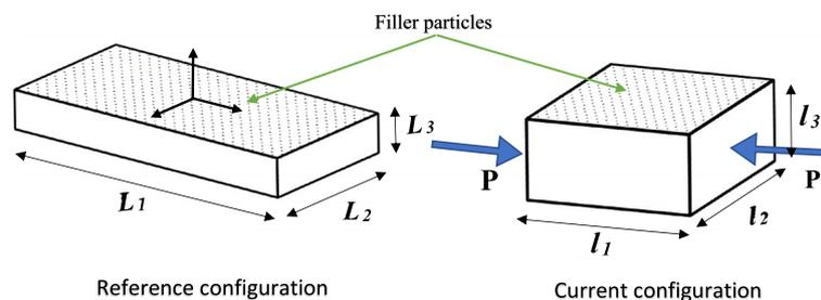
**Figure 1.** Schematic diagram of a rubber sample with filler particles in undeformed and deformed configurations.
