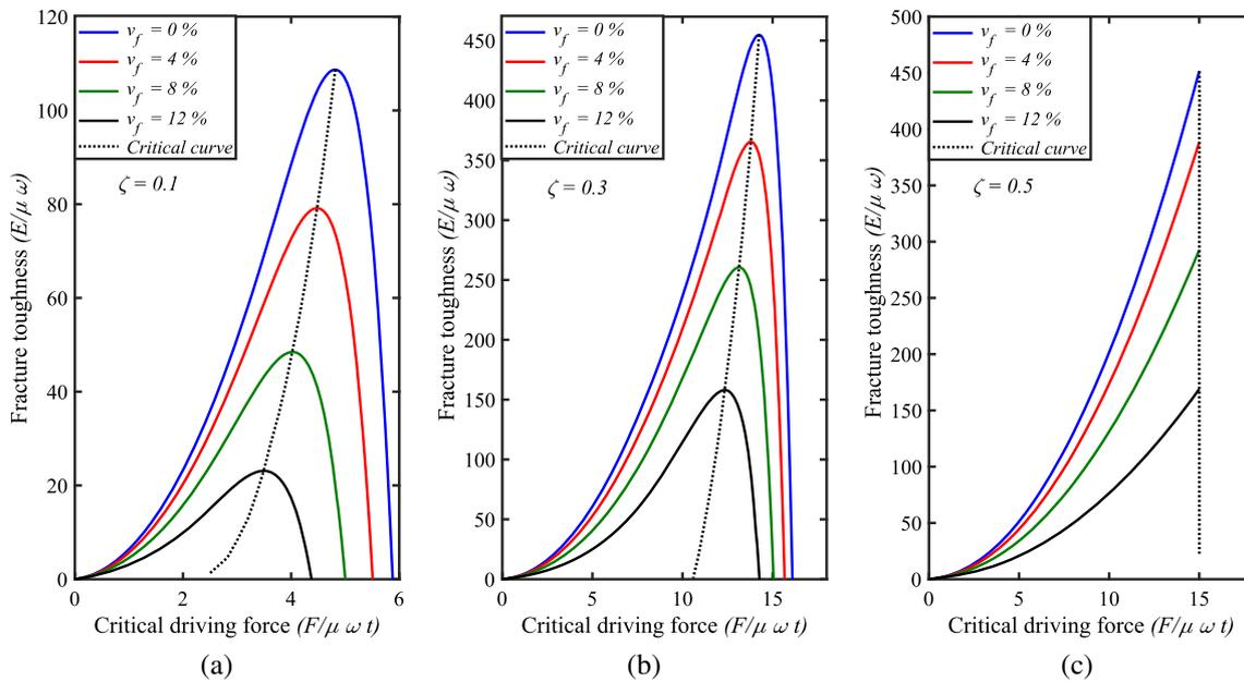
**Figure 9.** Fracture toughness versus critical driving force at different volume fractions of filler particles  $v_f$  for a fixed cut position (a)  $\zeta = 0.1$ , (b)  $\zeta = 0.2$  and  $\zeta = 0.5$ .
