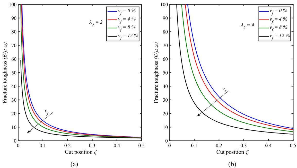
**Figure 8.** Fracture toughness versus cut position at different volume fractions of filler particles  $v_f$  for a fixed stretch (a)  $\lambda_2 = 2$  and (b)  $\lambda_2 = 4$  in leg 2.
