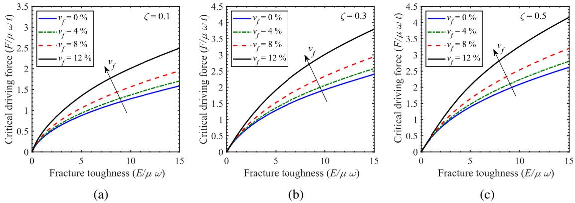
**Figure 7.** Critical driving force versus fracture toughness at different volume fractions of filler particles  $v_f$  for a fixed cut position (a)  $\zeta = 0.1$ , (b)  $\zeta = 0.3$ , and (c)  $\zeta = 0.5$ .
