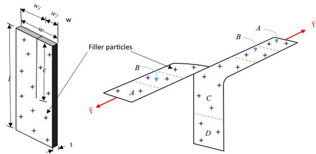
**Figure 4.** Schematic diagram of trousers test specimen.
