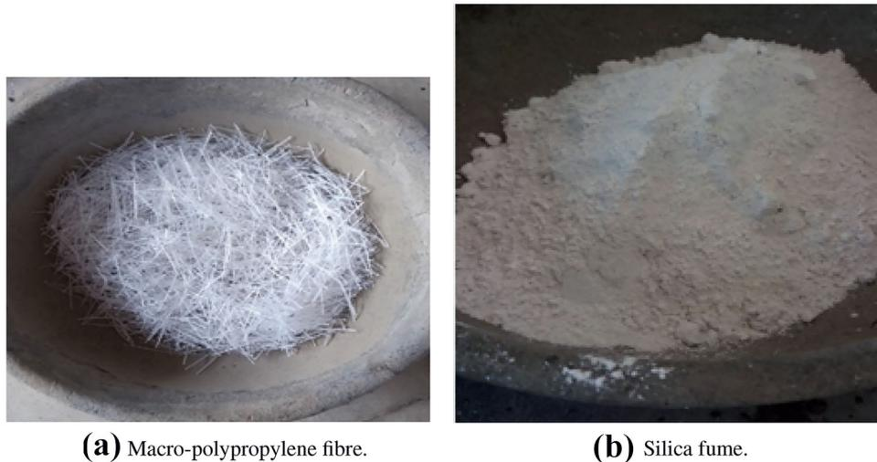
**Figure 1.** Photographs of materials used for preparation of concrete mix.
