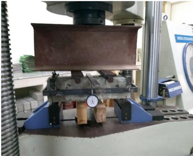
(b) Flexural strength test set-up.
