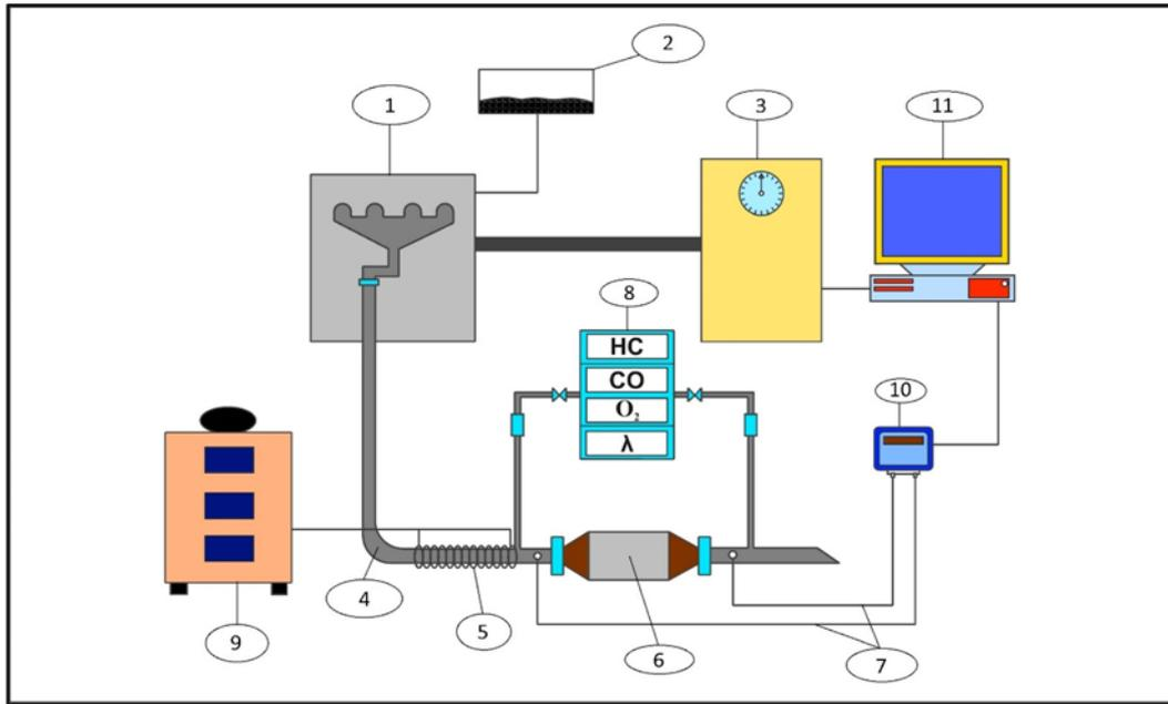
**Figure 1.** Schematic view of the experimental set-up. 1. Engine, 2. Fuel tank, 3. Dynamometer, 4. Exhaust Line, 5. Resistance, 6. Three-way catalytic converter 7. Thermocouples 8. Exhaust Gas Analyzer, 9. Voltage Adjustable Regulator (Three-phase variac), 10. Data logger 11. Computer.
