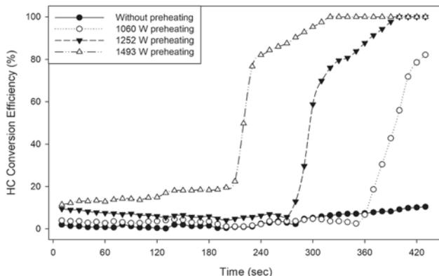
Figure 4. HC conversion efficiency of TWC at idle speed.
