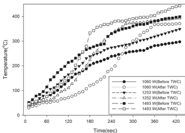
**Figure 2.** Temperature variation of before and after TWC at idle speed.
