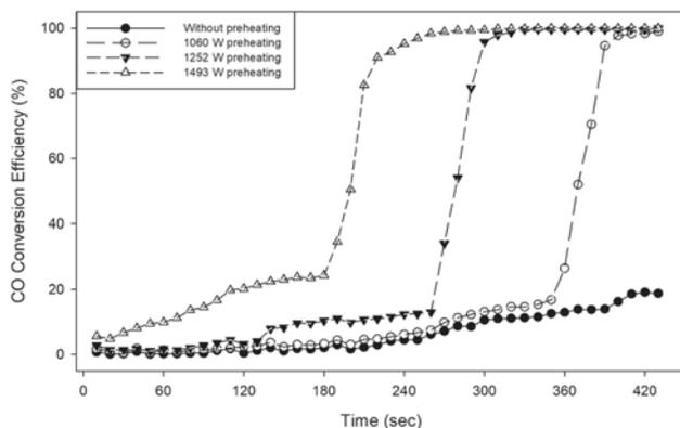
Figure 6. CO conversion efficiency of TWC at idle speed.
