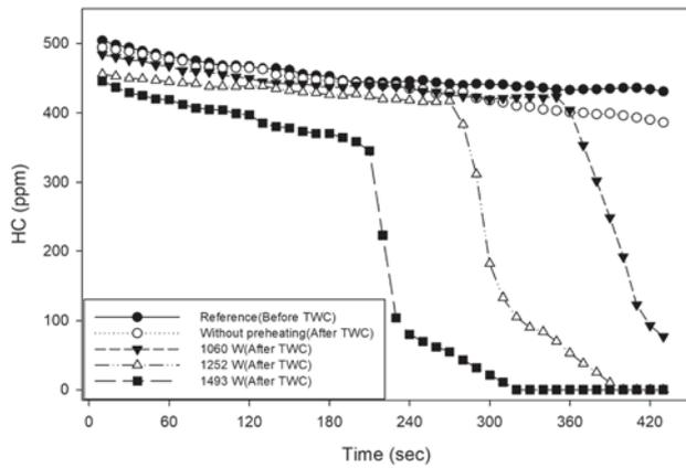
Figure 3. HC emission variation of TWC at idle speed.
