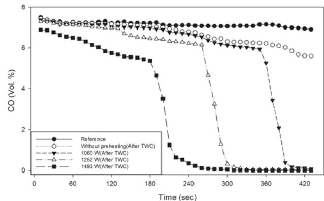
Figure 5. CO emission variation of TWC at idle speed.
