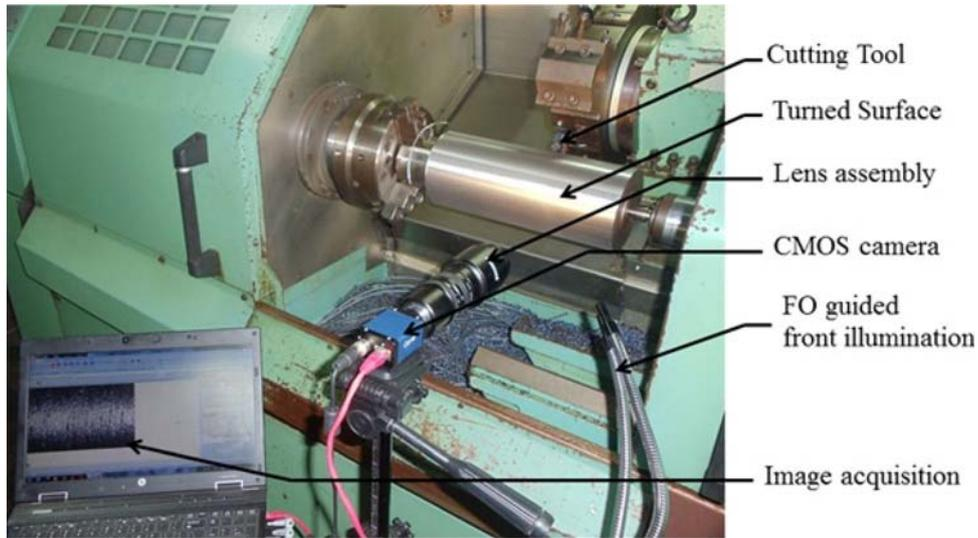
**Figure 1.** Experimental set-up for image acquisition.
