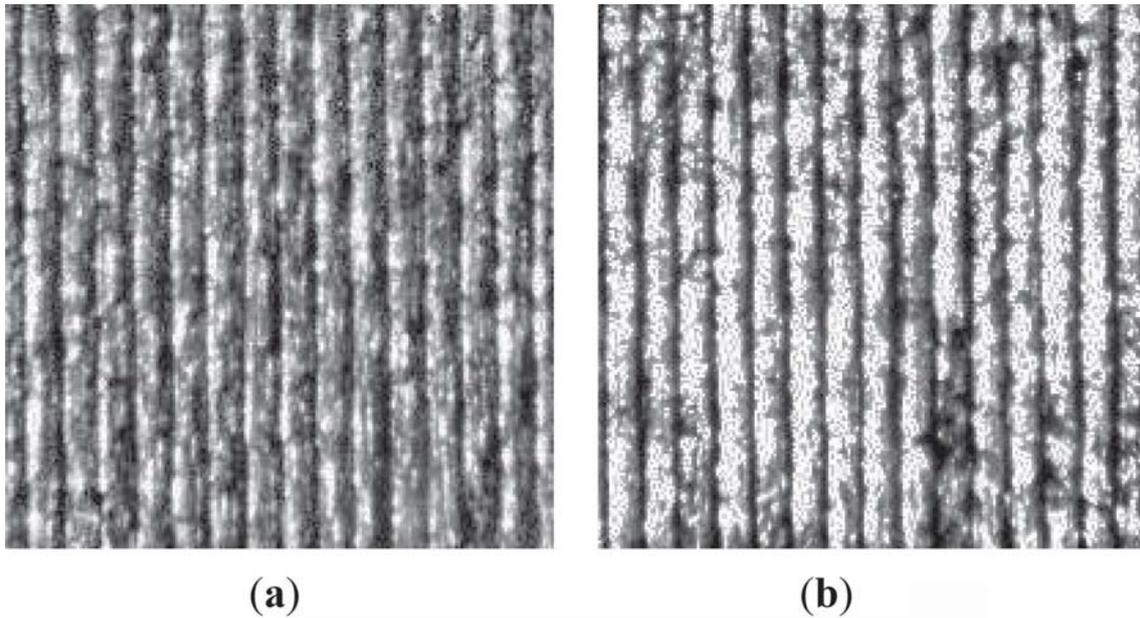
**Figure 4.** Turned surface images by (a) unworn tool, (b) worn tool using machining condition no. 5.
