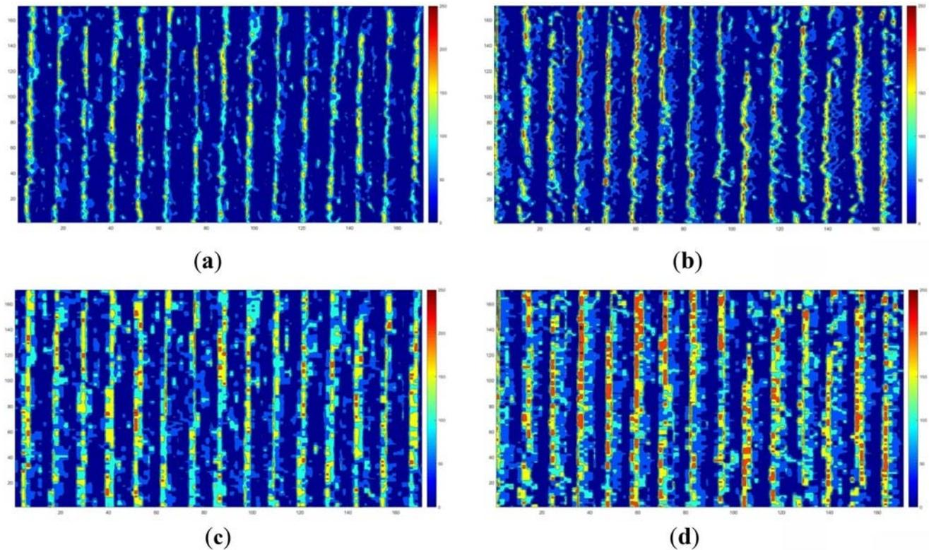
**Figure 6.** Contour maps of one of the filtered outputs for (a, b) 1st convolution layer, (c, d) 1st pooling layer, of figure 4a, b, respectively, analogous to gradient based image segmentation and DWT perspective.
