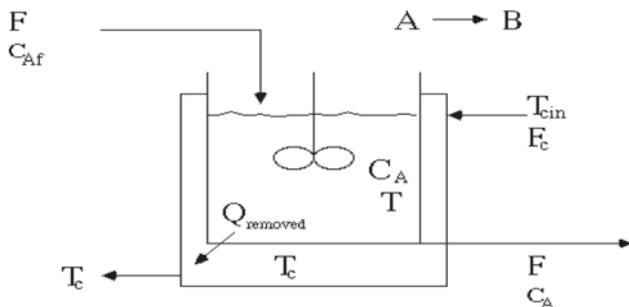
Figure 1. Schematic representation of Jacketed CSTR system.
