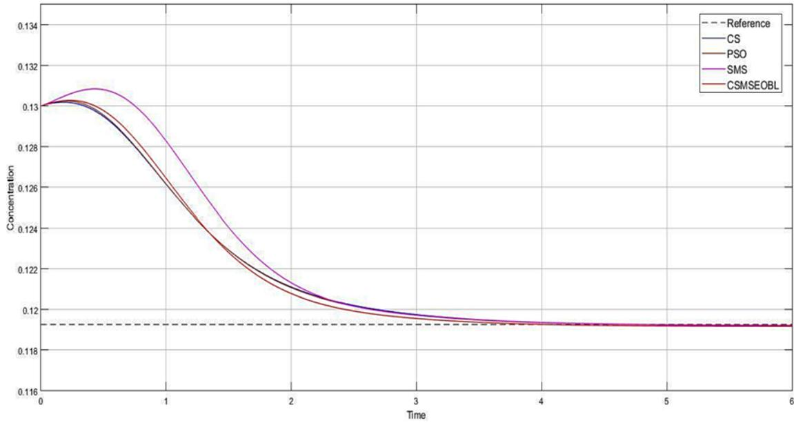
**Figure 6.** Comparison of concentration control of the CSTR system among different metaheuristic algorithms.
