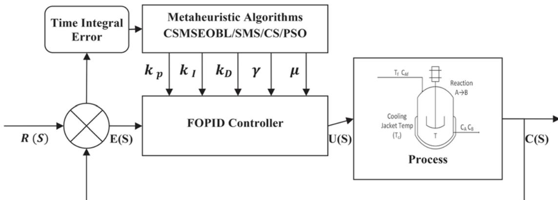
**Figure 3.** Optimized FOPID for Control of CSTR.
