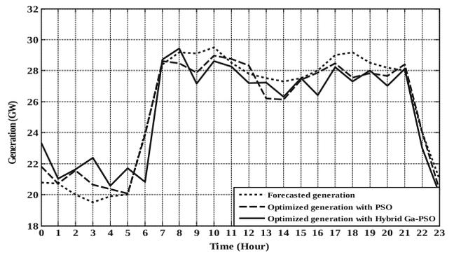
Figure 4. Optimized conventional generation pattern of a typical day with PSO and hybrid GA-PSO.
