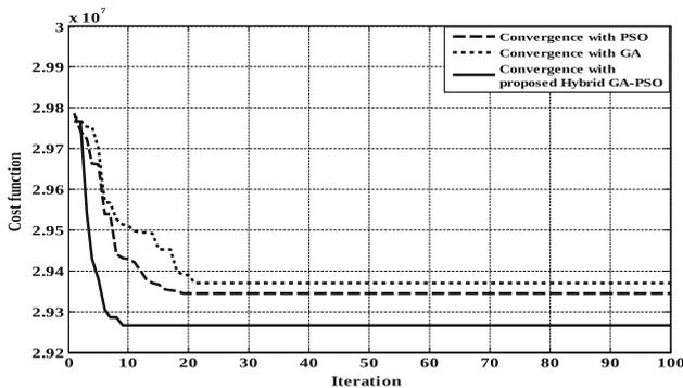
**Figure 6.** Cost convergence characteristics with different optimization algorithms.
