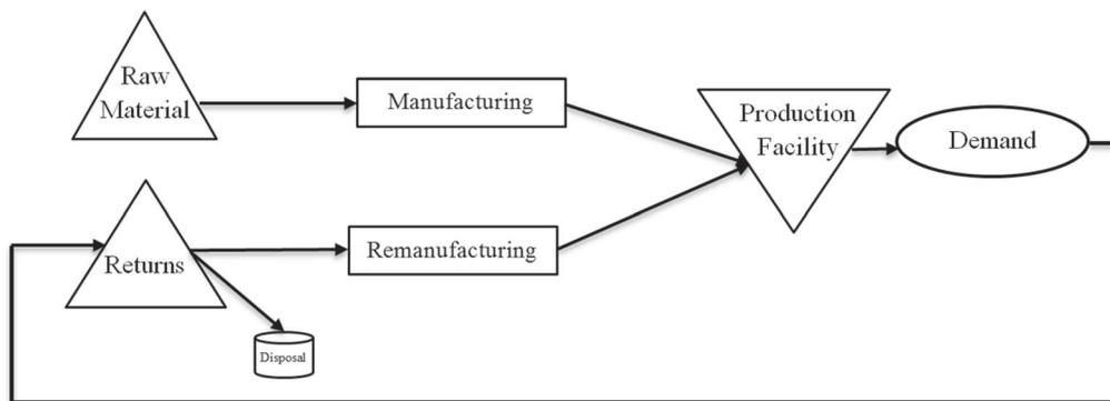
Figure 1. Hybrid manufacturing–remanufacturing system with a common demand stream.
