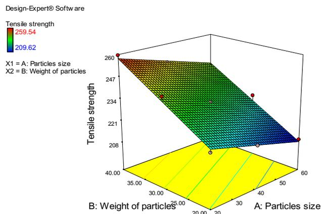
**Figure 2.** Surface plot for tensile strength corresponding to weight of particles versus particles size.
