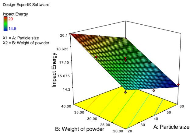
Figure 6. Surface plot for impact energy corresponding to weight of particles versus particles size.
