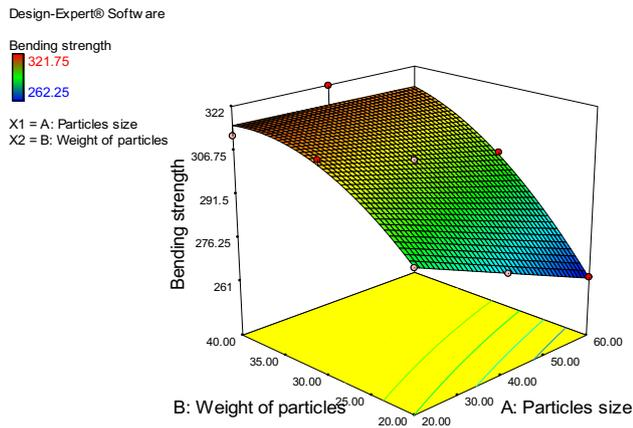
**Figure 4.** Surface plot for bending strength corresponding to weight of particles versus particles size.
