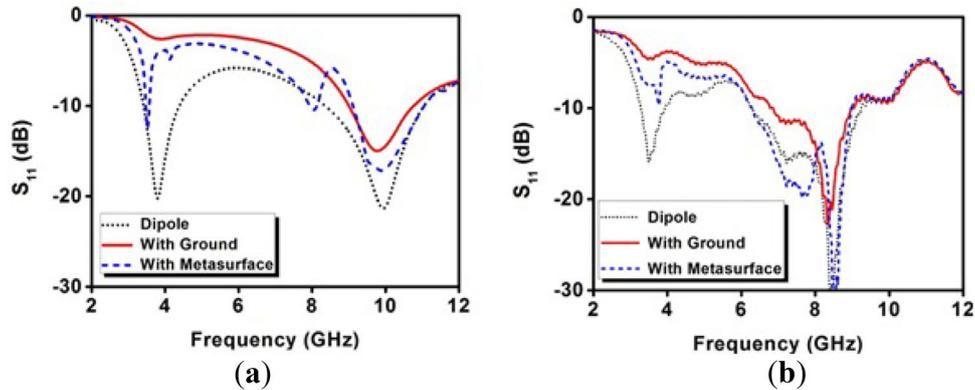
Figure 5. Reflection coefficient of dipole antenna with QBTR metasurface: (a) simulated and (b) measured.
