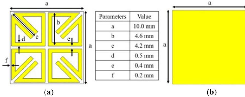
Figure 1. QBTR unitcell: (a) top layer and (b) bottom layer.
