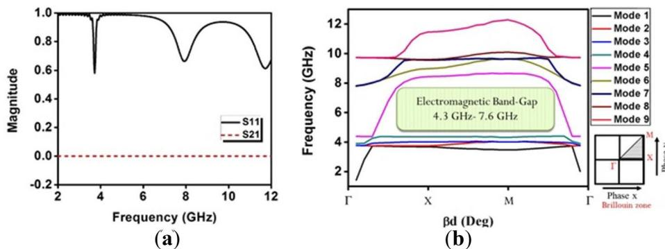
Figure 2. Simulated (a)  $S$ -parameter and (b) dispersion diagram.
