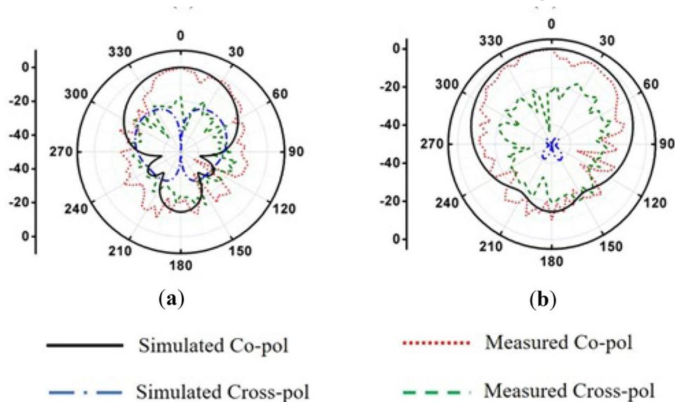
**Figure 7.** Radiation pattern of dipole antenna with QBTR metasurface at 6 GHz: (a)  $\Phi = 0^\circ$  and (b)  $\Phi = 90^\circ$ .
