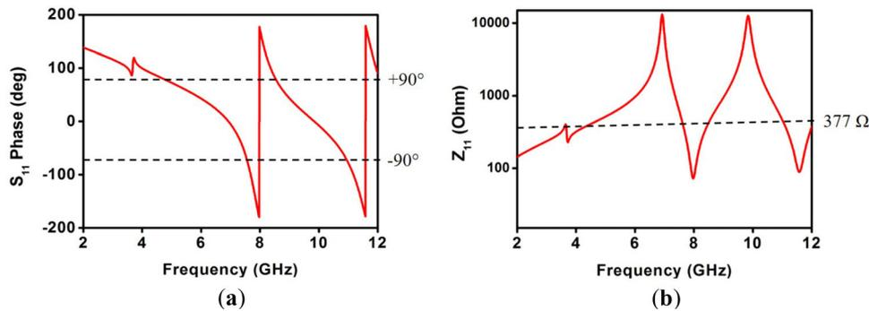
**Figure 3.** Simulated (a)  $S_{11}$  phase (deg) and (b)  $Z_{11}$  ( $\Omega$ ).
