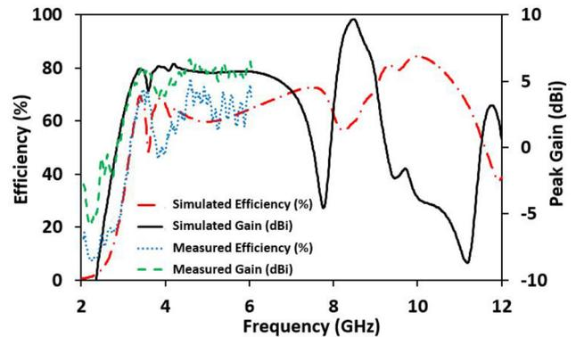
Figure 6. Efficiency (%) and peak gain (dBi) of dipole antenna with QBTR metasurface.
