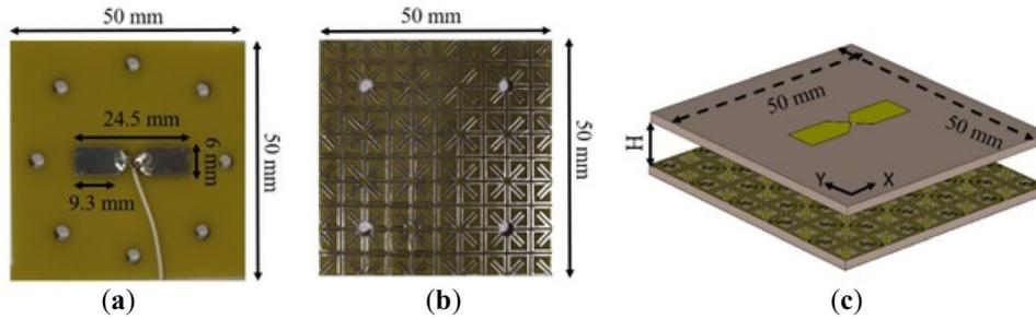
Figure 4. Fabricated prototype: (a) dipole antenna, (b) QBTR metasurface and (c) dipole assembly with QBTR metasurface.
