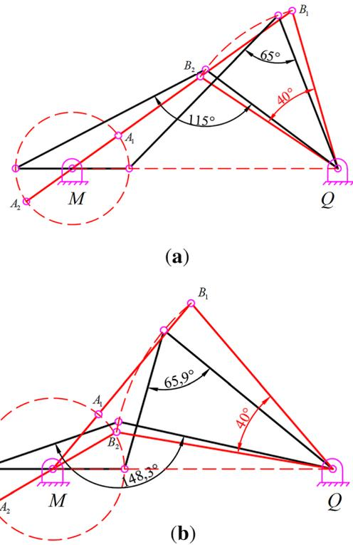
**Figure 6.** The crank–rocker mechanism and its limit positions obtained: (a) in case 8 and (b) in reference [21].
