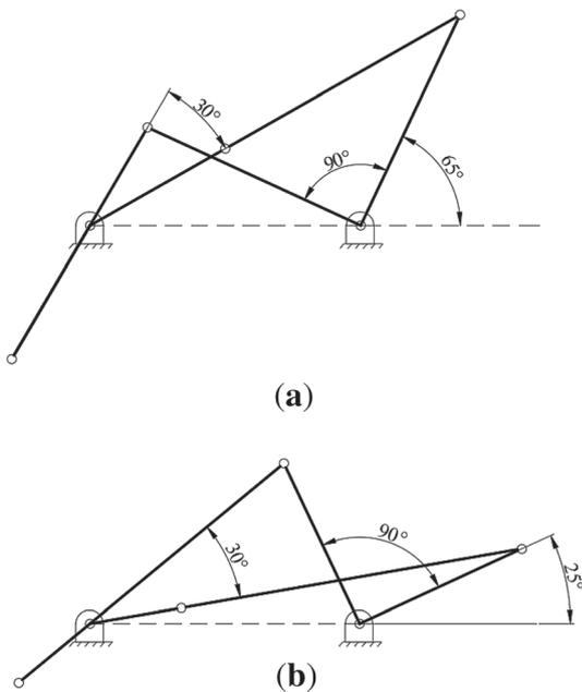
**Figure 3.** The crank-rocker mechanism and its limit positions obtained in case 2: (a) first solution and (b) second solution.
