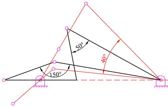
**Figure 7.** The crank-rocker mechanism of a maximum deviation from  $90^\circ$  equals  $60^\circ$  and a minimum deviation equals  $40^\circ$  with its limit positions obtained in case 8.
