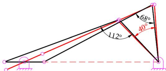
**Figure 8.** The crank-rocker mechanism maximum deviation from  $90^\circ$  equals  $22^\circ$  and its limit positions obtained in case 8.
