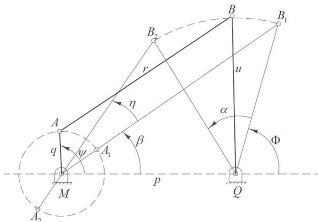
**Figure 1.** The parameters of the two limit positions and also the intermediate position of the crank–rocker mechanism.
