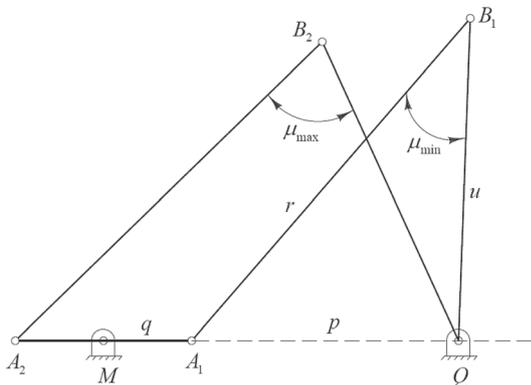
**Figure 2.** The minimum and maximum transmission angle configurations of crank–rocker mechanism.
