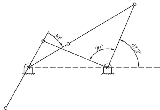
**Figure 5.** The crank-rocker mechanism and its limit positions obtained in case 7.
