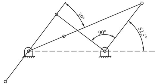
**Figure 4.** The crank-rocker mechanism and its limit positions obtained in case 3.
