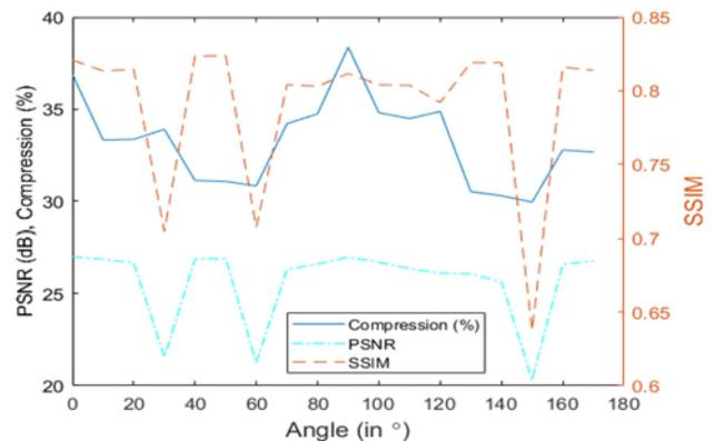
**Figure 10.** Effect of PSF orientation variation on compression metrics for the proposed method.
