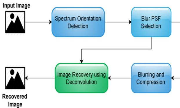
**Figure 1.** Flow diagram for the proposed spectrum-based compression method.
