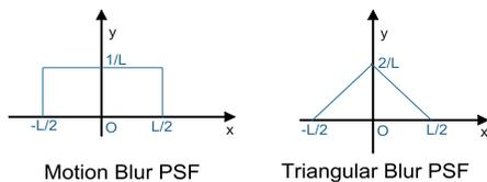
**Figure 3.** Motion blur PSF and triangular blur PSF.
