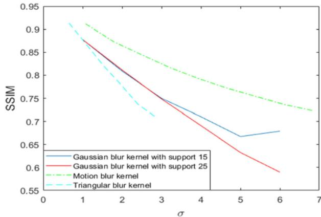
**Figure 6.** Effect of blur PSFs on SSIM.
