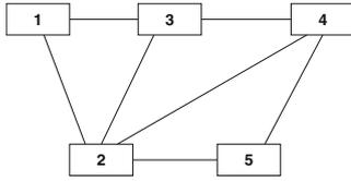
**Figure 1.** IEEE 5 bus system represented as a graph.
