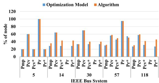
**Figure 5.** Percentage of nodes selected for PMU allocation.
