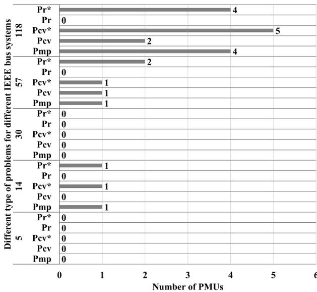
**Figure 3.** Summary of the difference in the number of PMUs allocated by the optimization model and Algorithm 1.
