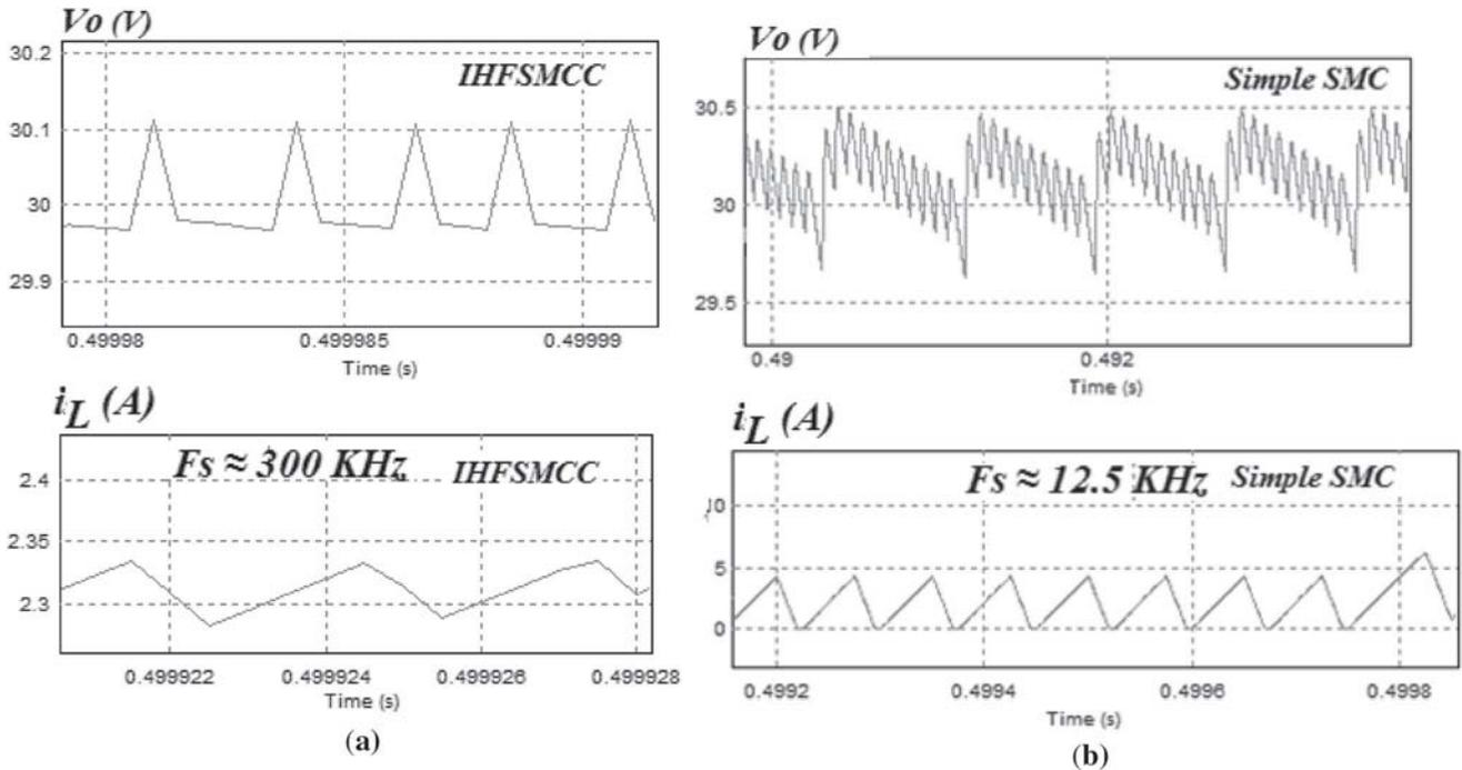
**Figure 9.** The magnified waveform of the current and voltage of the Boost converter for  $R = 48 \Omega$ ,  $E = 9V$ ,  $V_o = 30V$ ; (a)  $V_o = 35V$ ; (a) with the proposed IHFSMCC; (b) with the simple SMC.
