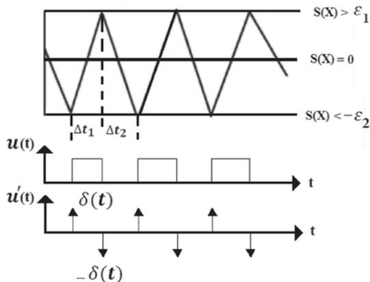
Figure 5. The sliding mode operation in CCM.
