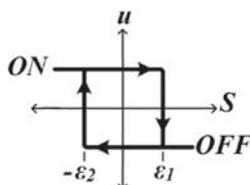
**Figure 3.** Figure illustrating the production of the hysteresis.
