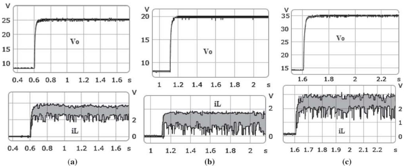
**Figure 11.** The transient response of the inductor current and output voltage of the converter with the IHFSMCC for  $R = 48 \Omega$ ; (a)  $E = 9$  V and  $V_O = 25$  V; (b)  $E = 9$  V and  $V_O = 20$  V; (c)  $E = 15$  V and  $V_O = 35$  V; (d)  $E = 18$  V and  $V_O = 35$  V
