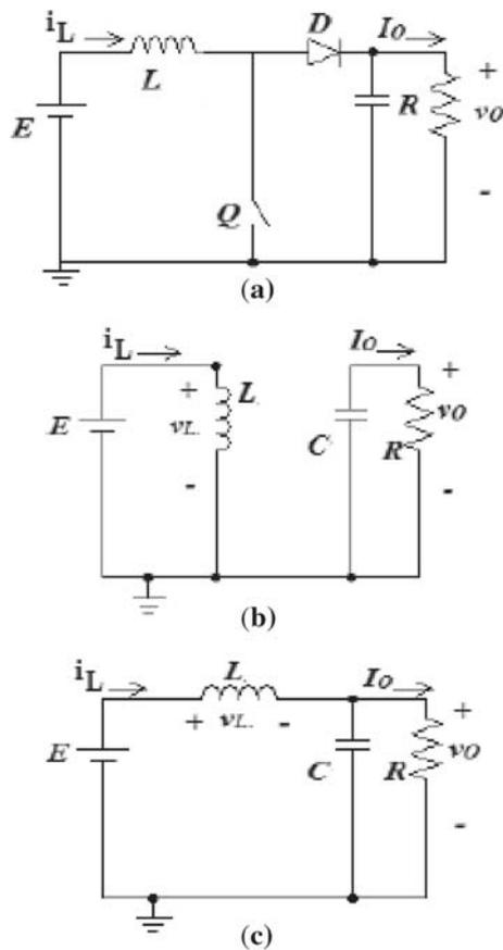
**Figure 1.** The CCM operation of a typical Boost converter; (a) the converter diagram; (b) the converter during switch-ON state; (c) the converter during switch-OFF state.
