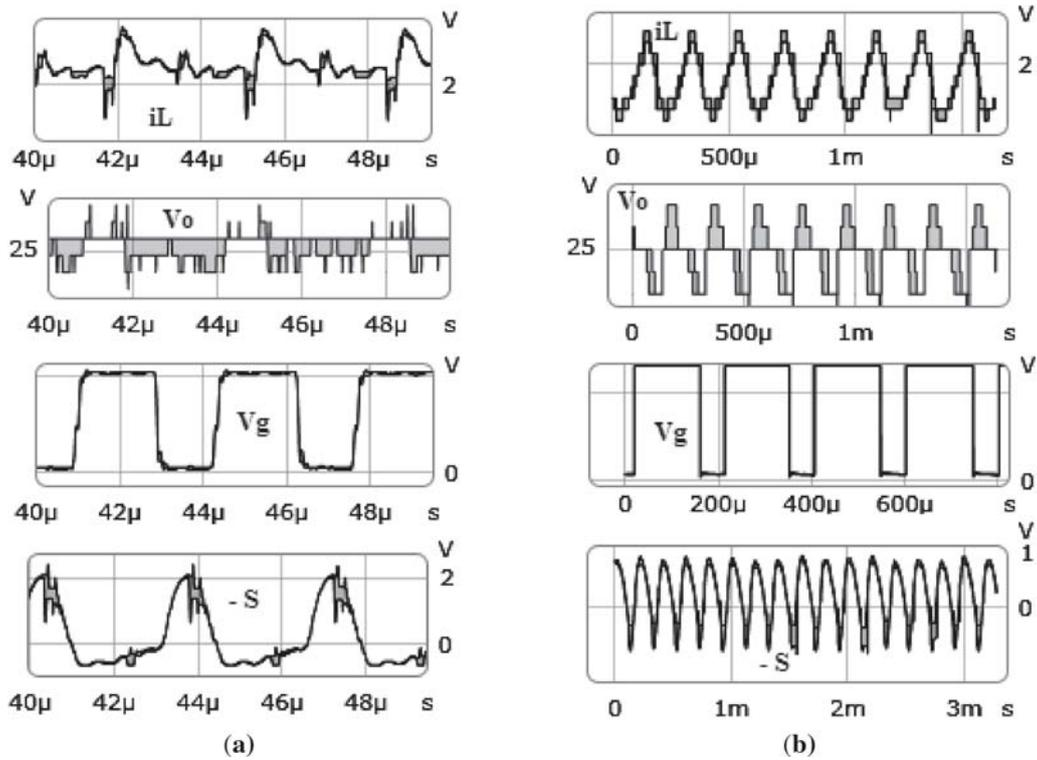
**Figure 14.** Voltage response in steady region for  $R = 48 \Omega$ ,  $V_O = 25 \text{ V}$  and  $E = 9 \text{ V}$ ; (a) The conventional SMC; (b) The proposed IHFSMCC.
