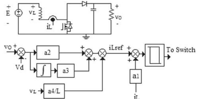
Figure 2. The general control scheme bandwidth.
