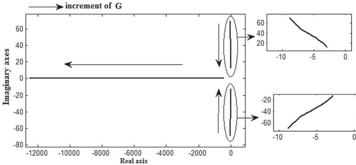
Figure 4. Root locus criterion for the developed system,  $R = 48 \Omega$ ,  $L = 0.00033 \text{ H}$ ,  $C = 0.0001 \text{ F}$ ,  $G > 1$ .
