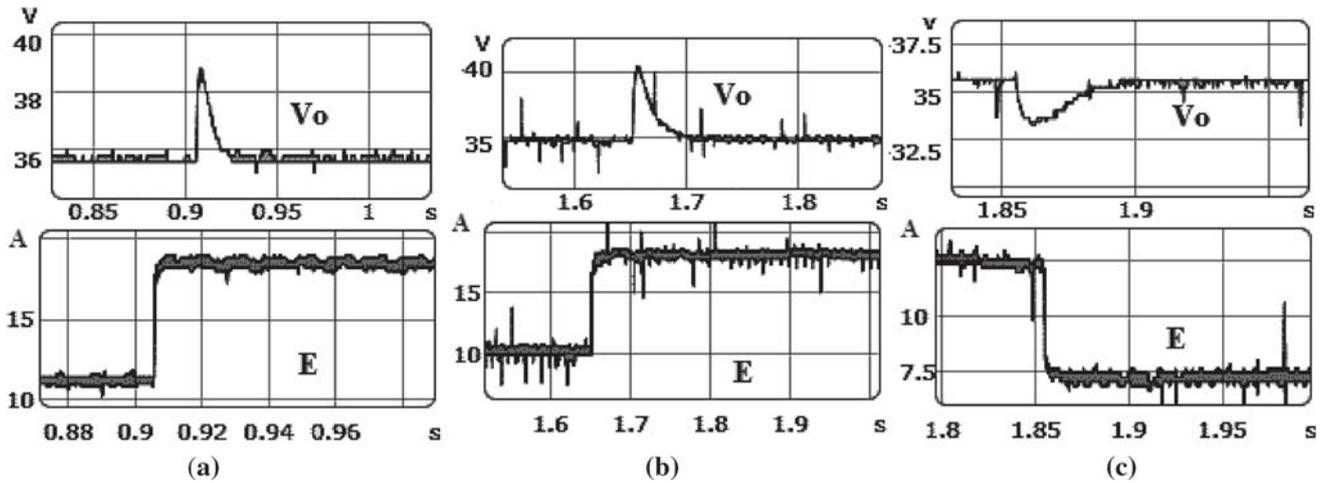
**Figure 12.** Responses of the output voltage for  $V_O=35$  V and input voltage variations; (a)  $R=96 \Omega$ ,  $E=11$  to  $18$  V; (b)  $R=36 \Omega$ ,  $E=10$  to  $18$  V; (c)  $R=96 \Omega$ ,  $E=12$  to  $7.5$  V.
