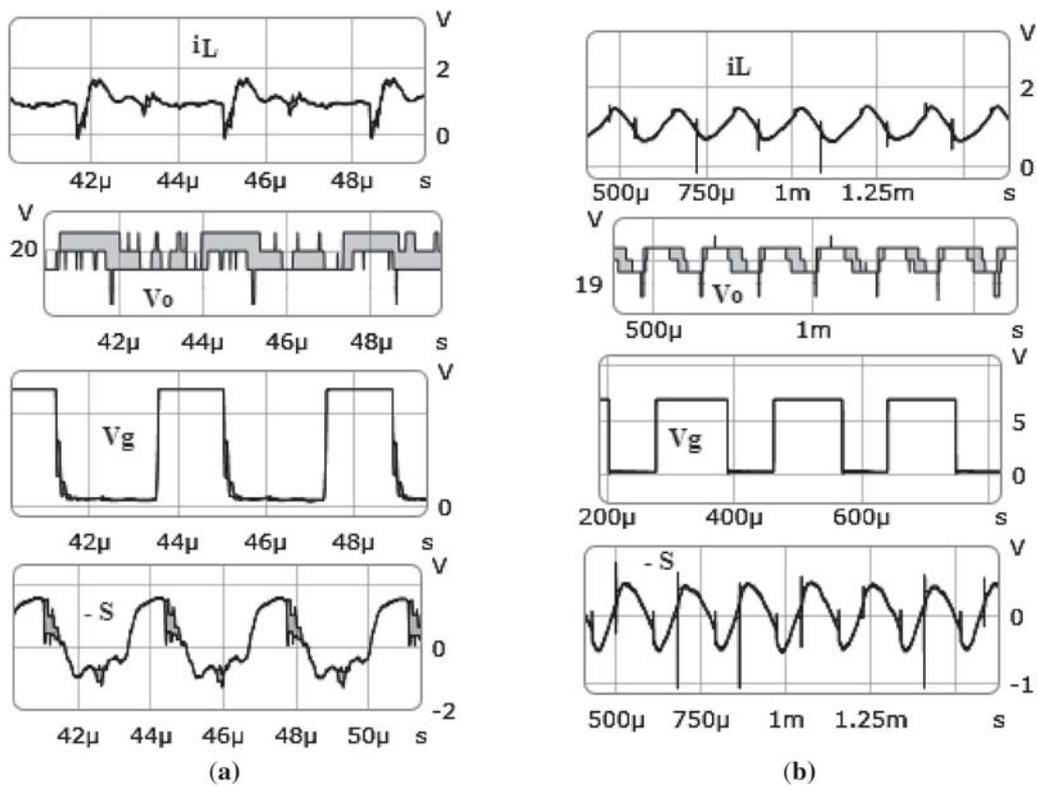
**Figure 15.** Voltage response in steady region for  $R = 48 \Omega$ ,  $V_O = 20 \text{ V}$  and  $E = 9 \text{ V}$ ; (a) The conventional SMC; (b) The proposed IHFSMCC.
