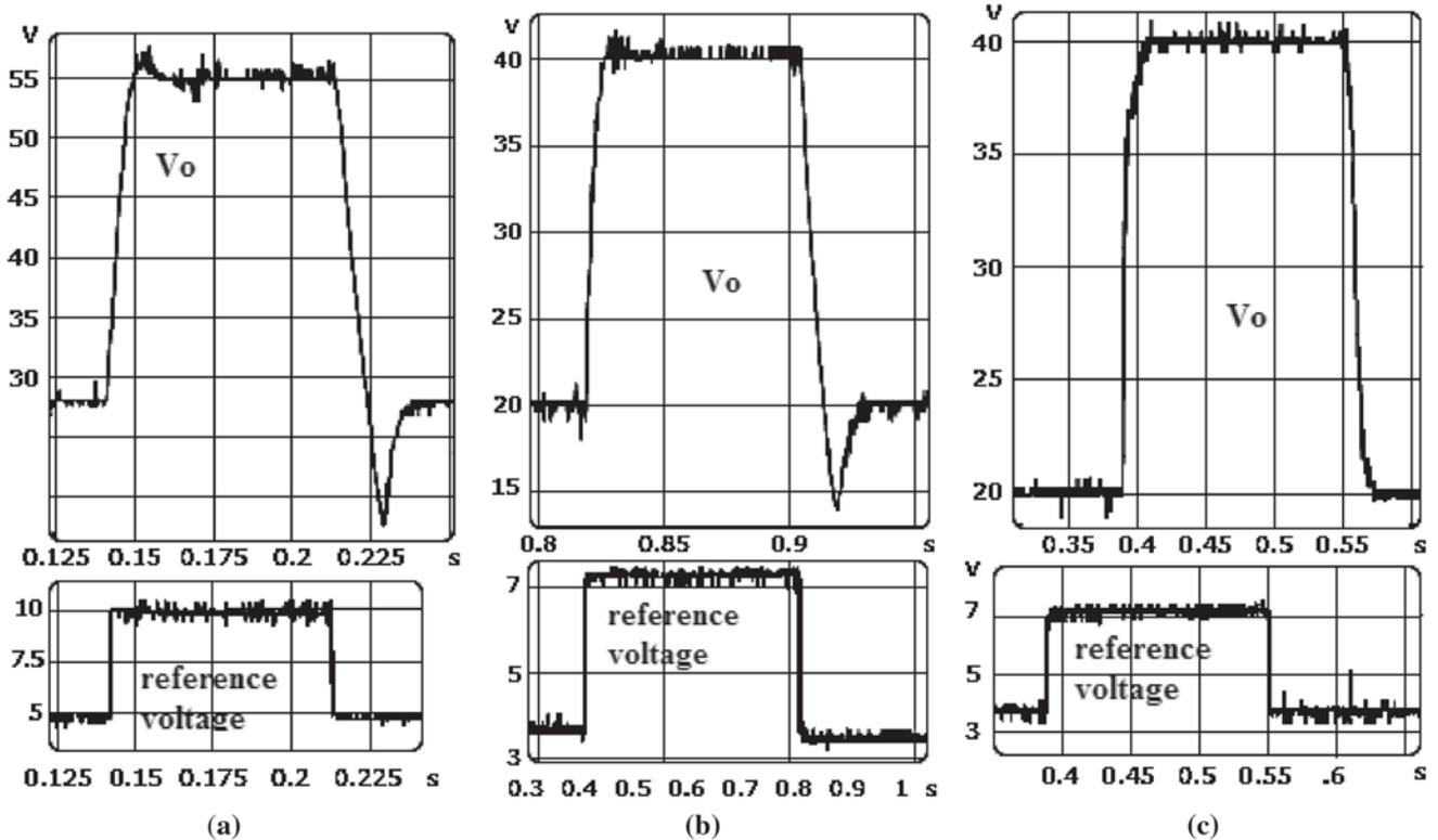
**Figure 13.** Voltage response against the voltage reference change; (a)  $E=12$  V,  $R=96 \Omega$  and  $V_O = 27$  V to  $55$  V; (b)  $E=12$  V,  $R = 96 \Omega$  and  $V_O = 40$  to  $20$  V; (c)  $E = 12$  V,  $R = 36 \Omega$  and  $V_O = 20$  V to  $40$  V.
