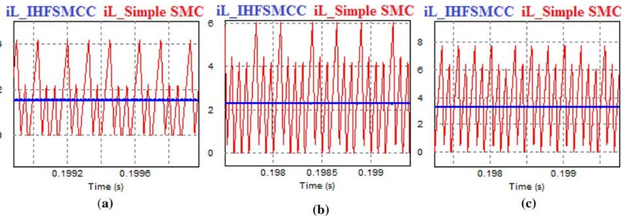
**Figure 8.** The instantaneous waveform of the input current of the Boost converter under the proposed IHFSMCC and simple SMC for  $R = 48 \Omega$ ,  $E = 9 \text{ V}$ ; (a)  $V_o = 25 \text{ V}$ ; (b)  $V_o = 30 \text{ V}$ ; (c)  $V_o = 35 \text{ V}$ .
