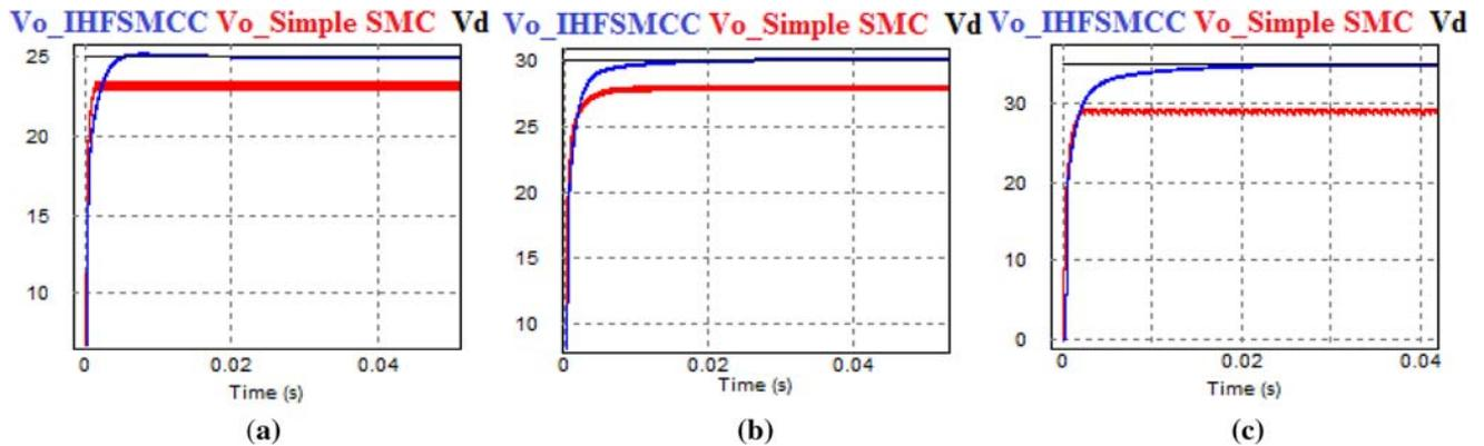
**Figure 7.** The simulated response of the input current and output voltage of the Boost converter with the proposed IHFSMCC and simple SMC for  $R = 48 \Omega$ ,  $E = 9 \text{ V}$ ; (a)  $V_d = 25 \text{ V}$ ; (b)  $V_d = 30 \text{ V}$ ; (c)  $V_d = 35 \text{ V}$ .
