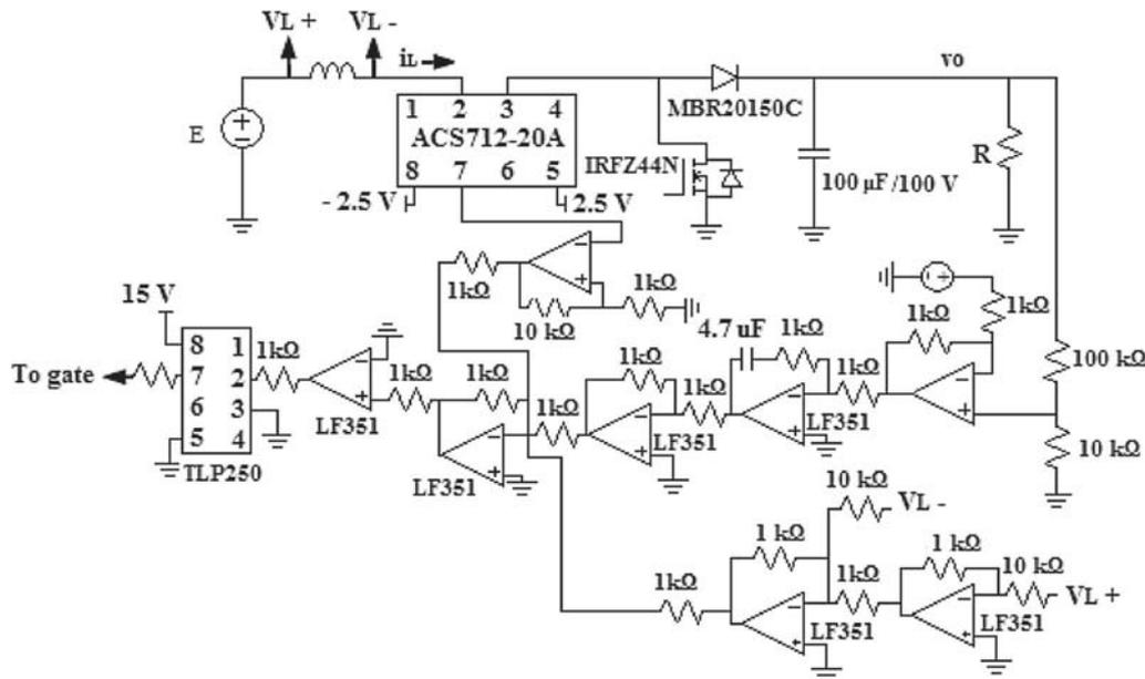
**Figure 10.** Basic structure of the Boost converter under the IHFSMCC in analogue platform.
