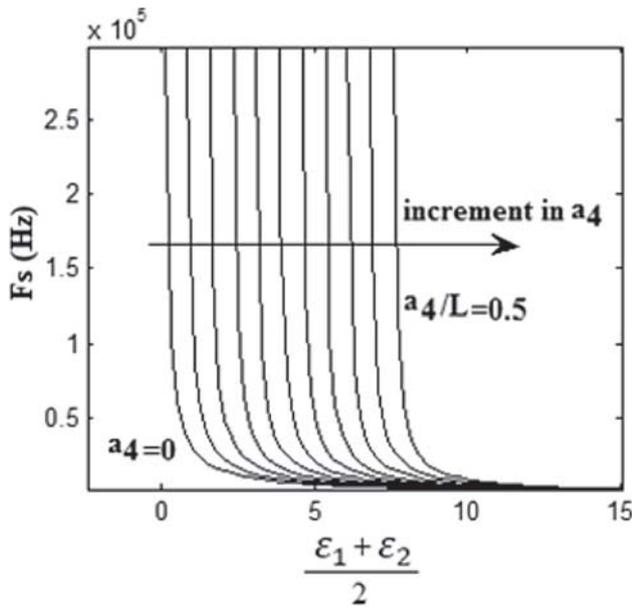
**Figure 6.** The converter frequency with the proposed IHFSMCC for  $V_d = 30$  V,  $R = 48 \Omega$ ,  $E = 9$  V and different values of  $a_4$ .
