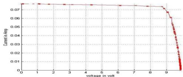
Figure 2. I-V characteristics of a solar module at 500 W/m<sup>2</sup> by using a variable resistor.
