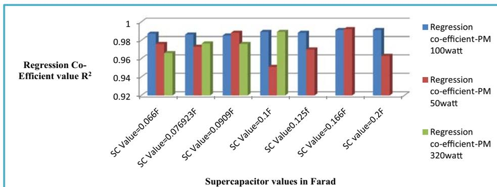
Figure 6. Regression co-efficient of  $P_m$  values against different supercapacitor ratings.
