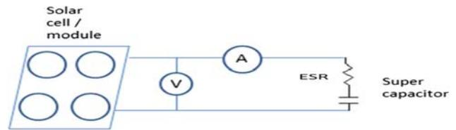
Figure 1. I-V characterization using supercapacitor loading.
