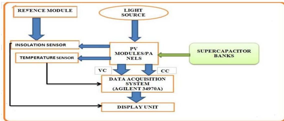
**Figure 4.** Functional blocks of the testing set-up.
