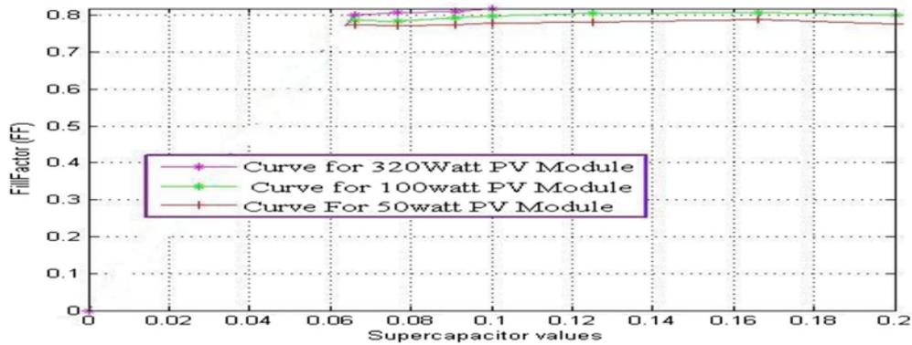
**Figure 7.** Fill Factor vs. supercapacitor values for different poly-Si PV modules.
