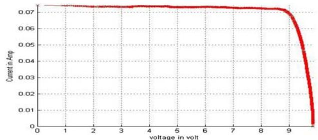
Figure 3. I-V characteristics of a solar module at 500 W/m<sup>2</sup> by using a supercapacitor.
