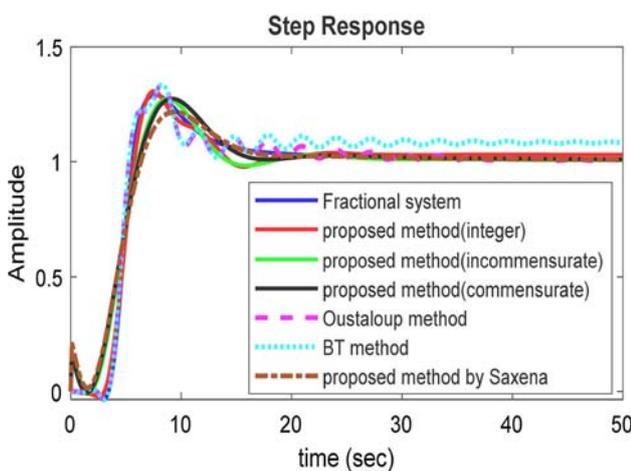
**Figure 7.** Step response of non-minimum fractional order system and their approximations.
