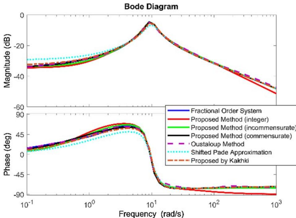
**Figure 5.** Comparison of frequency response of fractional order system and famous reduction methods by the proposed reduced order models approximation.
