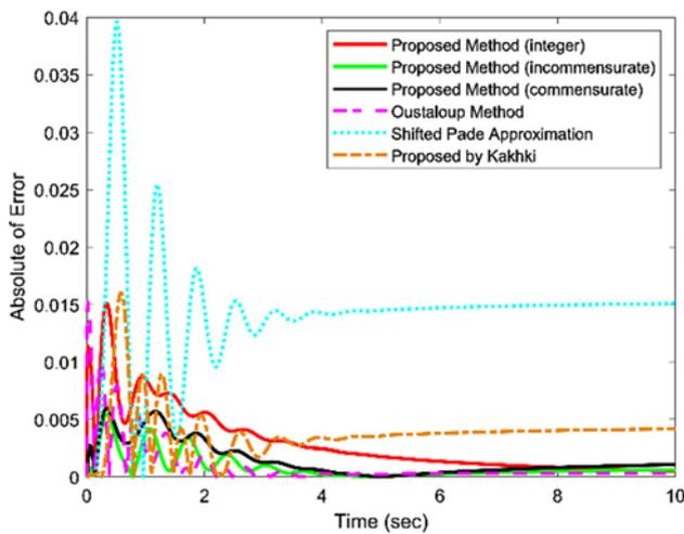
**Figure 6.** Time evolution of absolute error of various methods for test system 1.
