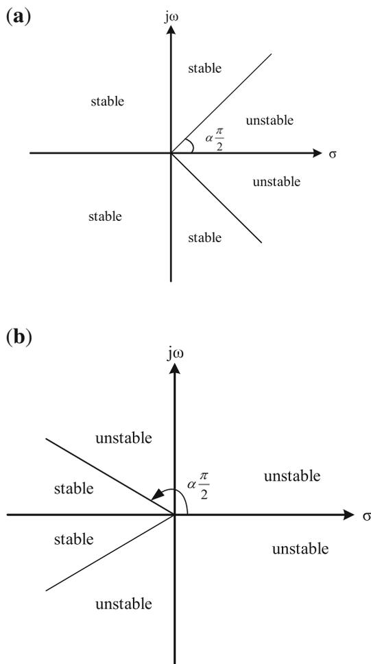
**Figure 1.** (a) Stability region of fractional order LTI system with order  $0 \leq \alpha \leq 1$ . (b) Stability region of fractional order LTI system with order  $1 \leq \alpha \leq 2$ .
