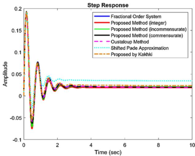
**Figure 4.** Comparison of step response of fractional order system and famous reduction methods by the proposed reduced order models approximation.
