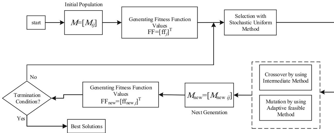
**Figure 2.** Procedure of employed genetic algorithm.
