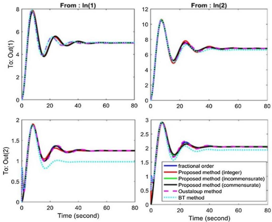
**Figure 9.** Step response of MIMO fractional order system and their approximations.
