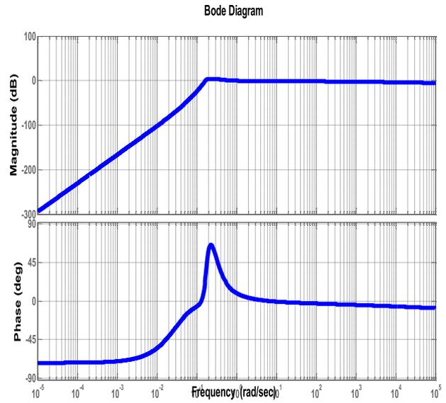
**Figure 2.** Bode plot of sensitivity of heating furnace using primary controller.
