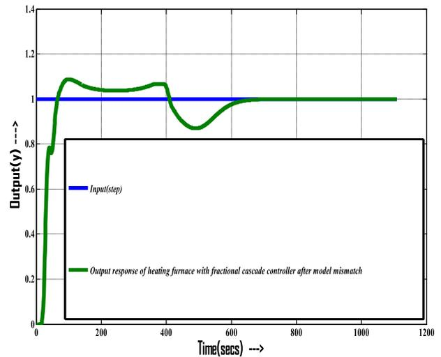
**Figure 3.** Output response of heating furnace after model mismatching.
