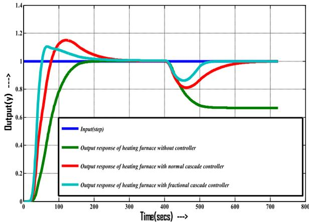
**Figure 1.** Output response of heating furnace by FO-PID cascade controller.
