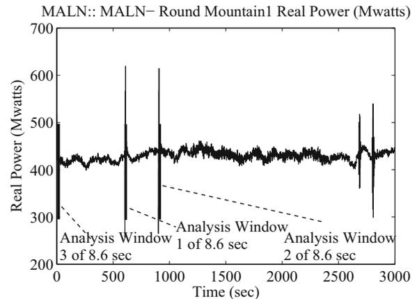
**Figure 3.** Probing data corresponding to flow of power.
