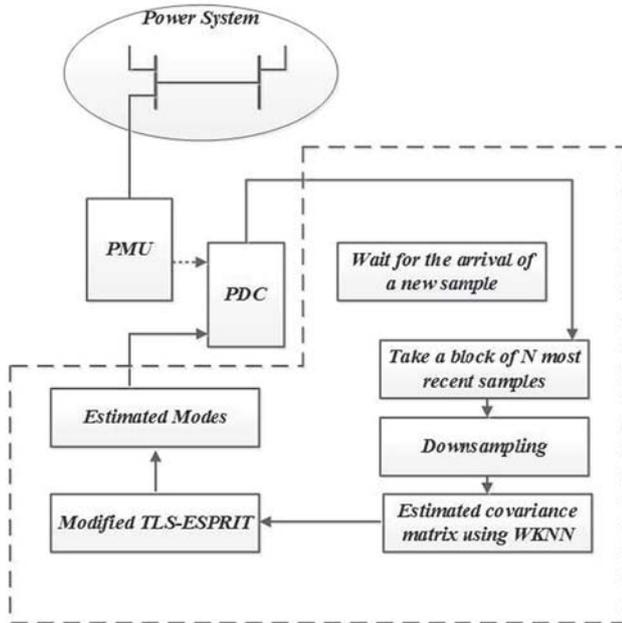
**Figure 1.** Block diagram of the proposed WKNN-TLS-ESPRIT scheme.
