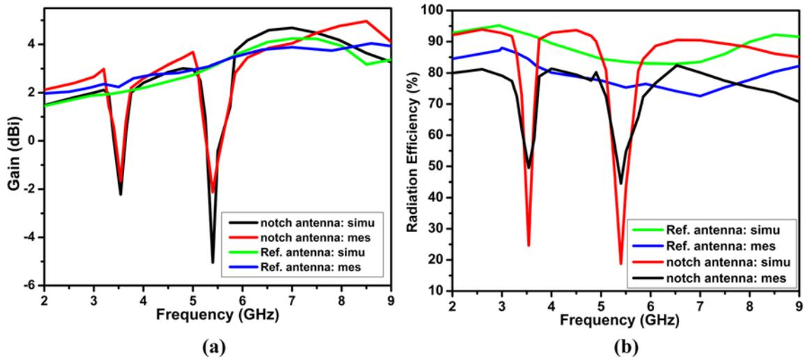
Figure 5. Simulated and measured (a) gain response and (b) radiation efficiency of reference and dual notched antennas.
