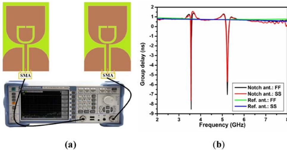
Figure 6. (a) Group delay and transfer function ( $S_{21}$ ) measurement set-up in side-by-side orientation and (b) group delay comparison plots for reference antenna and proposed filtenna.
