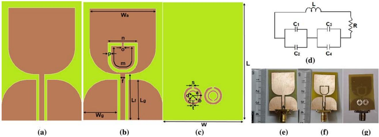
**Figure 1.** Schematic of (a) reference antenna, (b) top view and (c) bottom view of dual notched antenna, (d) equivalent circuit of circular split ring resonator, fabricated prototype of (e) reference antenna and (f) top view and (g) bottom view of filter antenna.
