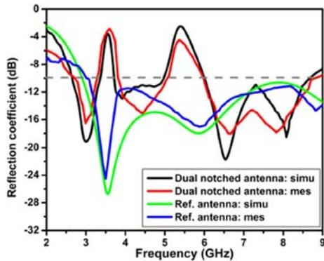
**Figure 2.** Comparison of simulated and measured reflection coefficients.
