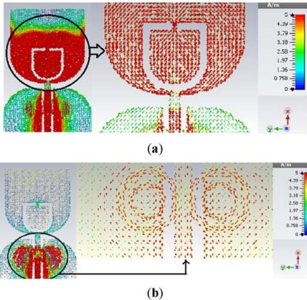
**Figure 3.** Simulated surface current of dual notched antenna at (a) 3.55 GHz and (b) 5.4 GHz.
