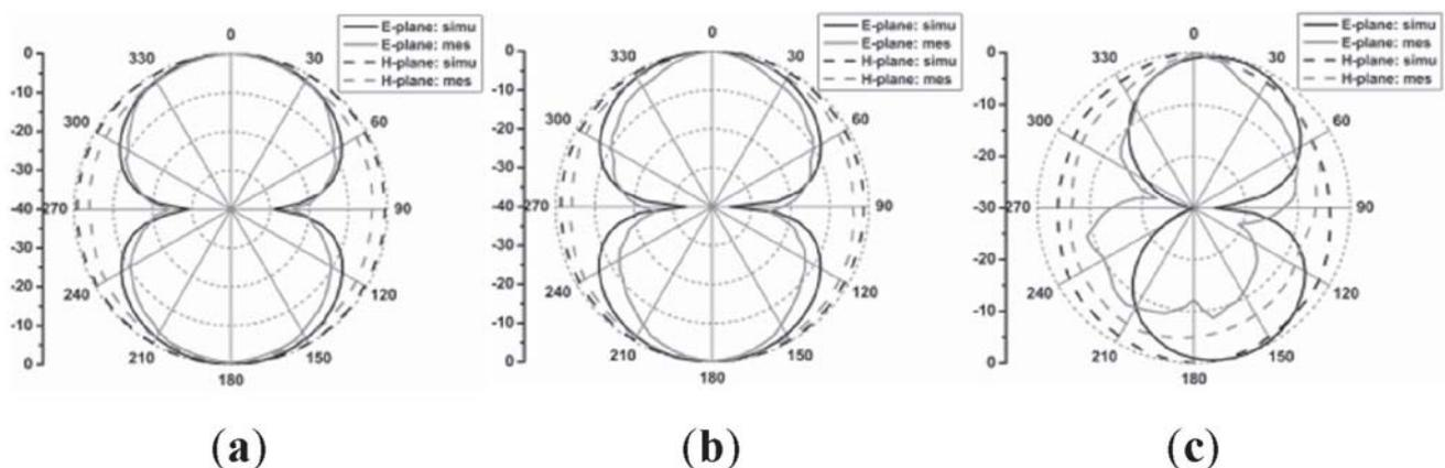
**Figure 4.** Simulated and measured co-polarized antenna radiation patterns at (a) 3 GHz, (b) 6.6 GHz and (c) 8 GHz.
