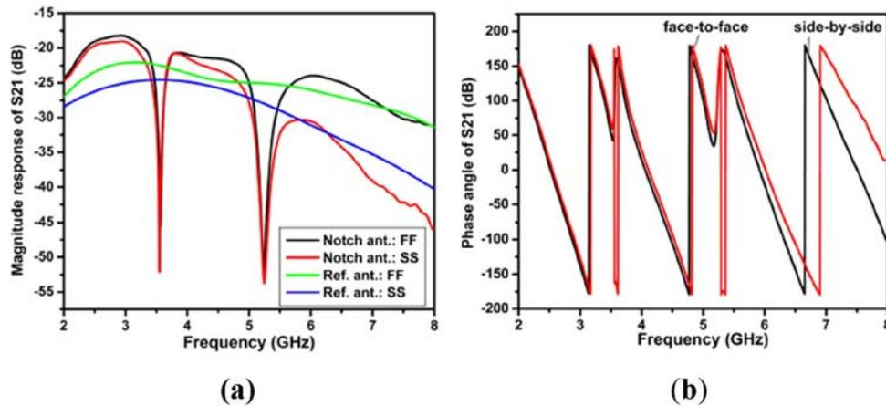
**Figure 7.** (a) Magnitude response of transfer function for reference antenna and filtenna. (b) Phase response of filtenna, in face-to-face and side-by-side orientations.
