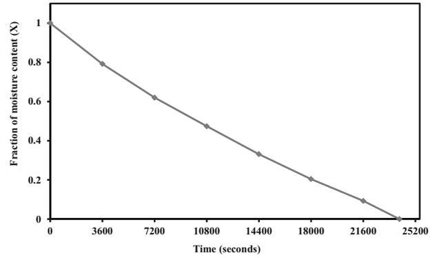
**Figure 9.** Variation of initial moisture content (X) during drying stage.
