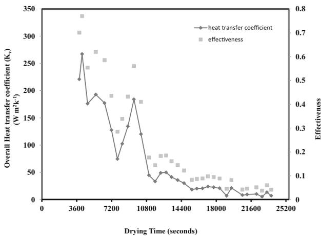
**Figure 12.** Determination of overall heat transfer coefficient ( $K_v$ ) and effectiveness in drying process—mini channel.
