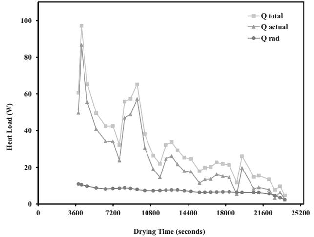
**Figure 11.** Determination of heat load in product during drying process.
