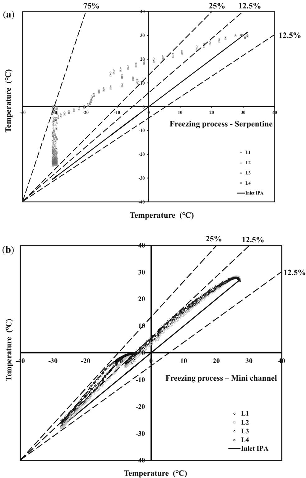
**Figure 4.** (a) Product temperature variation in freezing process—serpentine channel. (b) Product temperature variation in freezing process—mini-channel.
