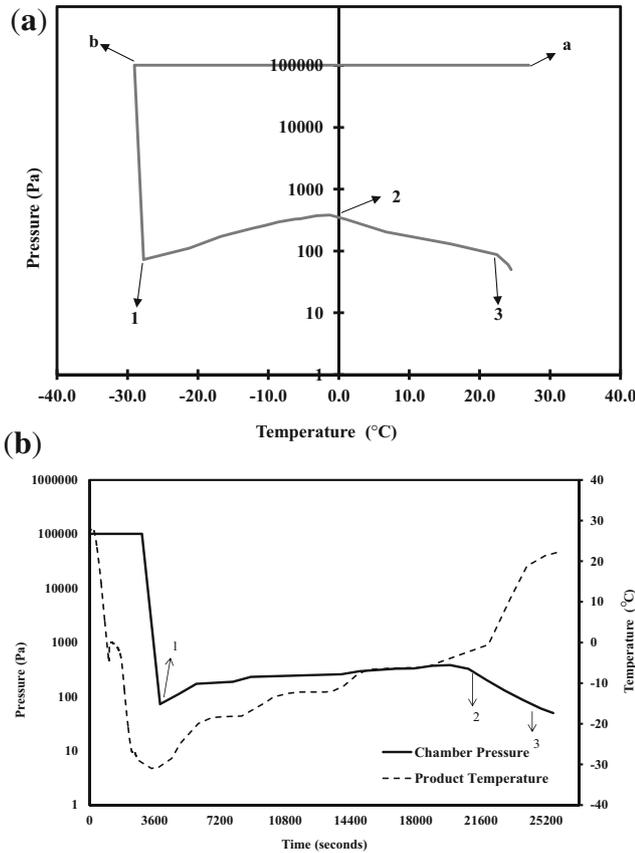
**Figure 8.** (a) Chamber Pressure against Product Temperature plot during drying process. (b) Chamber Pressure vs Product Temperature vs drying time.
