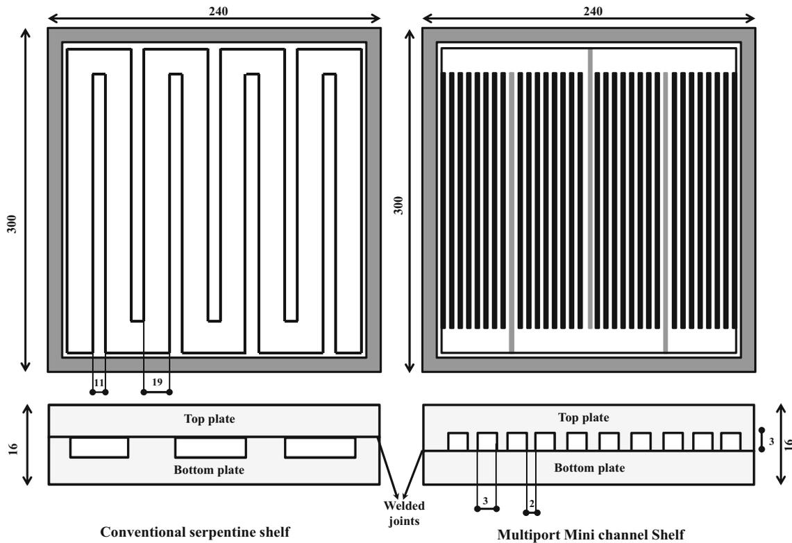
**Figure 2.** Conventional serpentine and proposed mini-channel shelf heat exchanger layout.
