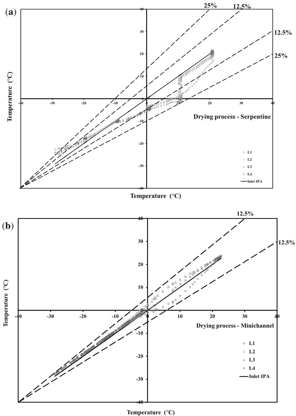
**Figure 5.** (a) Product temperature variation in drying process—serpentine channel. (b) Product temperature variation in drying process—mini-channel.
