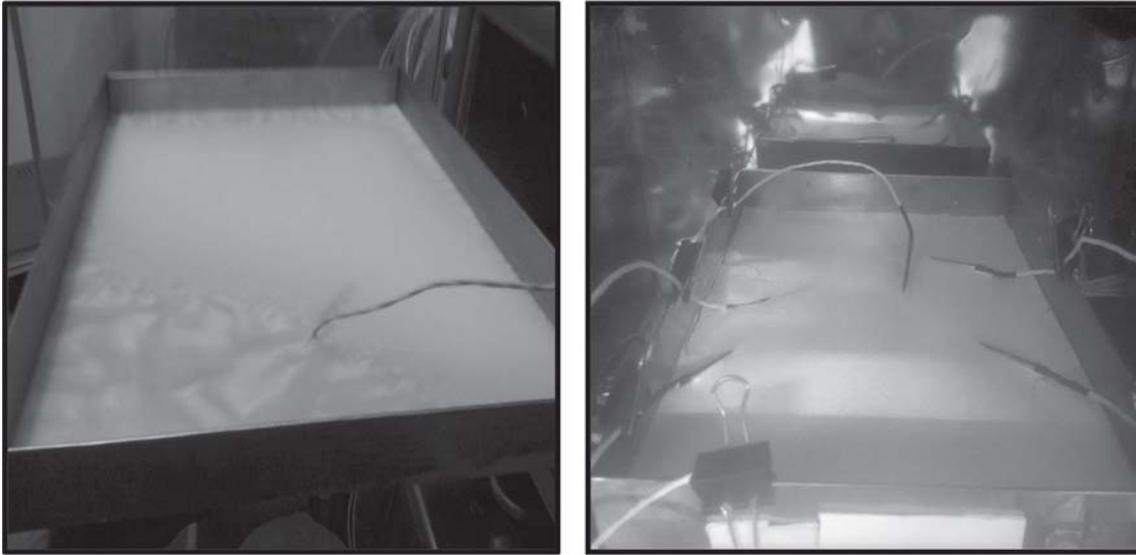
**Figure 6.** Ice layer uniformity in freezing stage—(a) serpentine, (b) mini channel.
