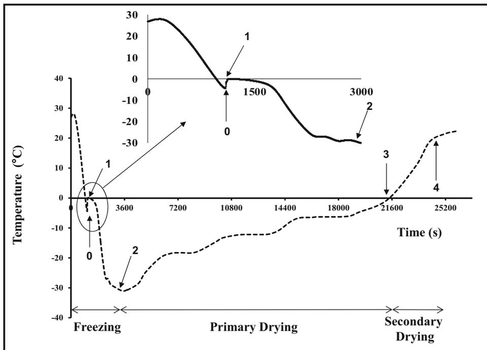
**Figure 7.** Cooling curve behavior in freezing process—mini channel.
