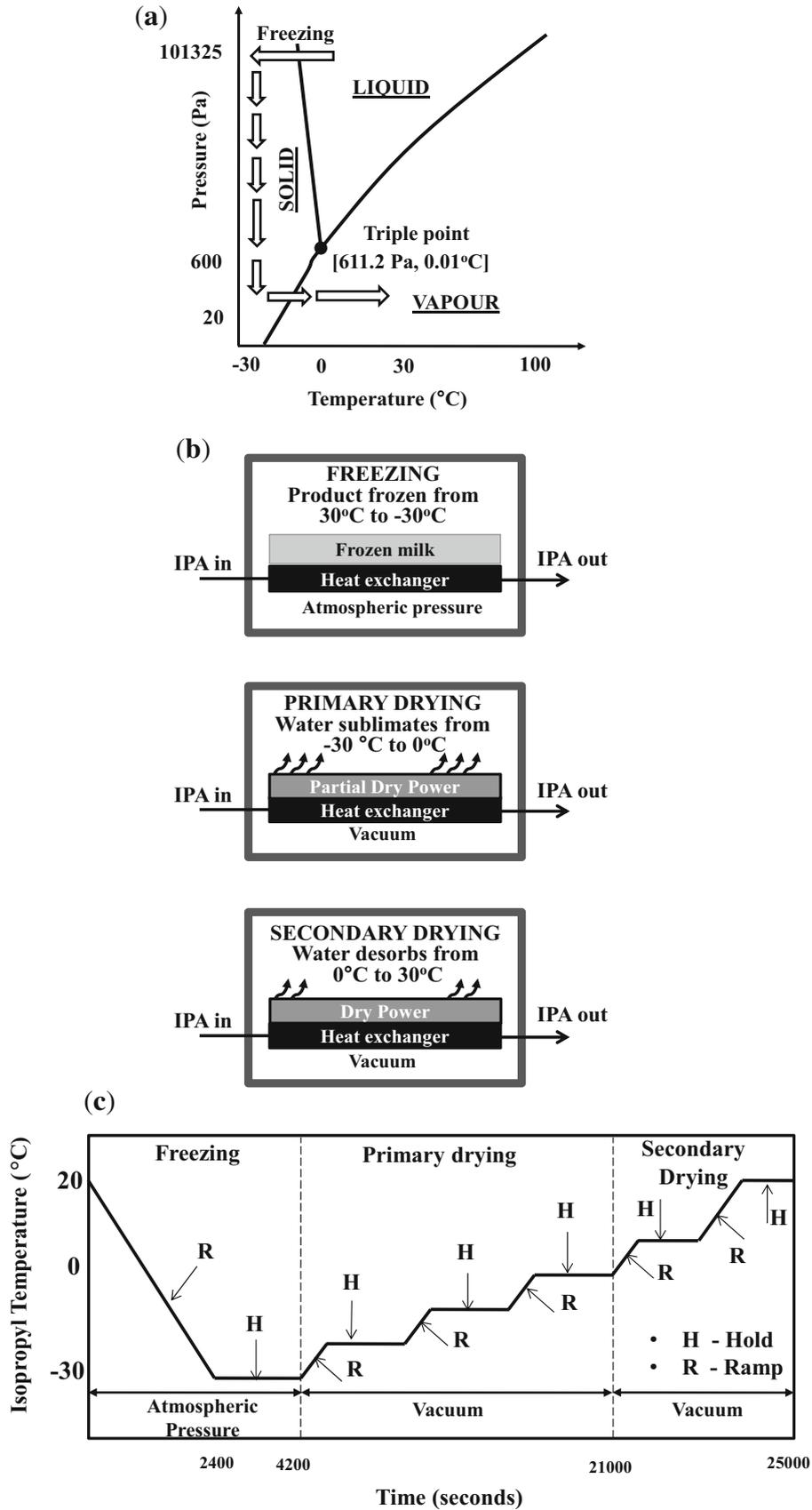
◀ **Figure 1.** (a) Pressure Temperature (PT) diagram of distilled water. (b) Different stages of Freeze drying process. (c) Ramping and holding sequence of isopropyl during drying process.
