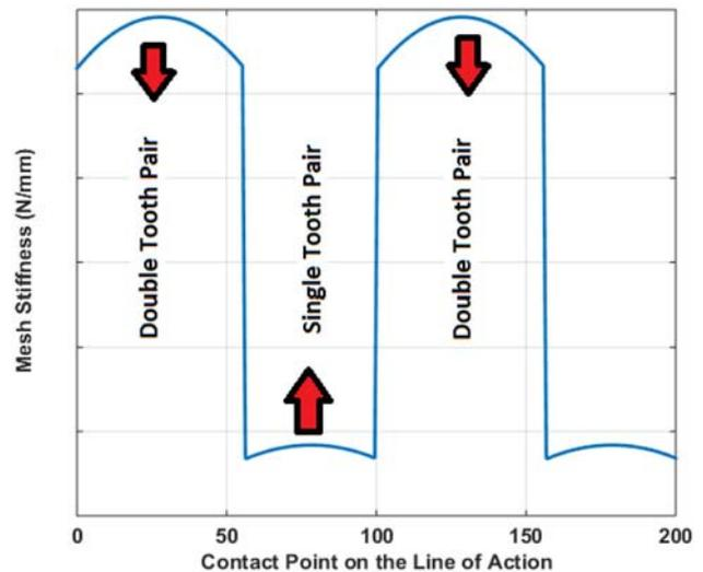
Figure 4. Mesh stiffness variation for one mesh cycle.
