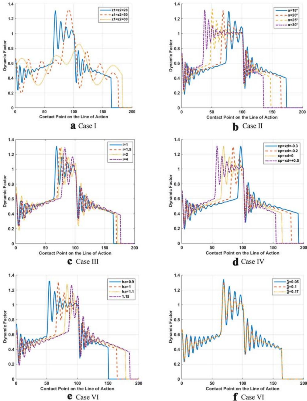
**Figure 8.** The effects of gear design parameters on dynamic loads for one mesh period. a)  $z_1, z_2$ : Teeth number, b)  $\alpha$ : Pressure angle, c)  $i$ : Reduction ratio, d)  $x_p, x_d$ : Profile shifting factor, e)  $h_a$ : Addendum factor, f)  $\zeta$ : Damping ratio.
