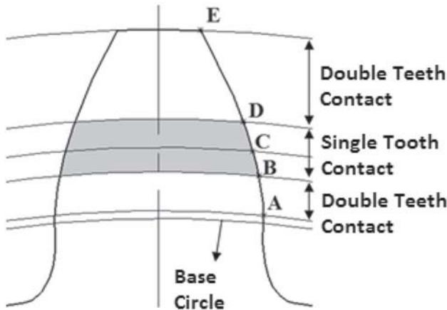
Figure 3. Single and double contact zones on the tooth profile.
