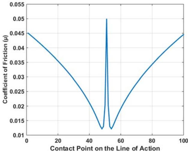
**Figure 6.** Change of coefficient of friction for one mesh cycle.
