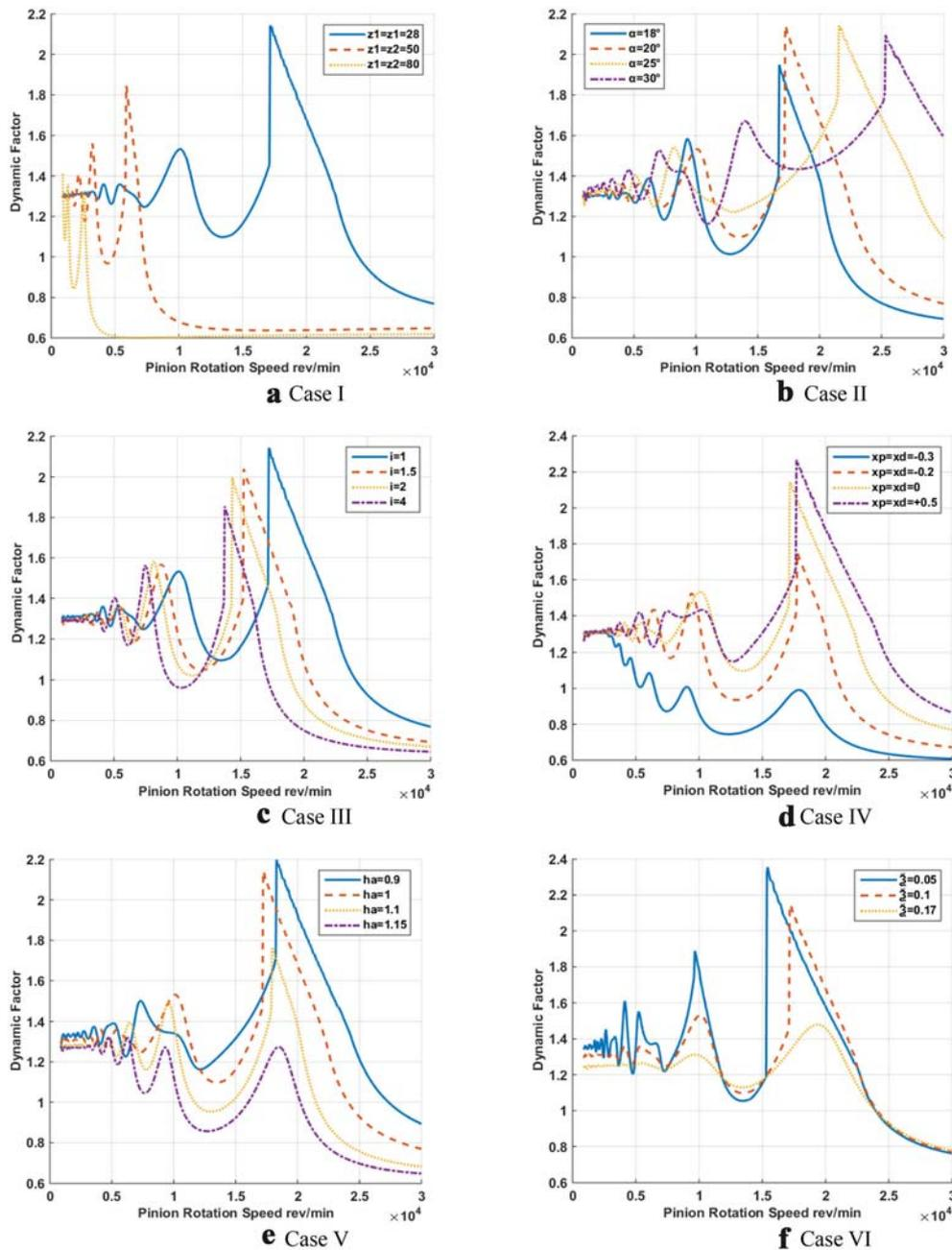
**Figure 9.** The effects of gear design parameters on dynamic factor between 400–30000 rpm. a)  $z_p, z_g$ : Tooth number, b)  $\alpha$ : Pressure angle, c)  $i$ : Reduction ratio, d)  $x_p, x_d$ : Profile shifting factor, e)  $h_a$ : Addendum factor, f)  $\zeta$ : Damping ratio.
