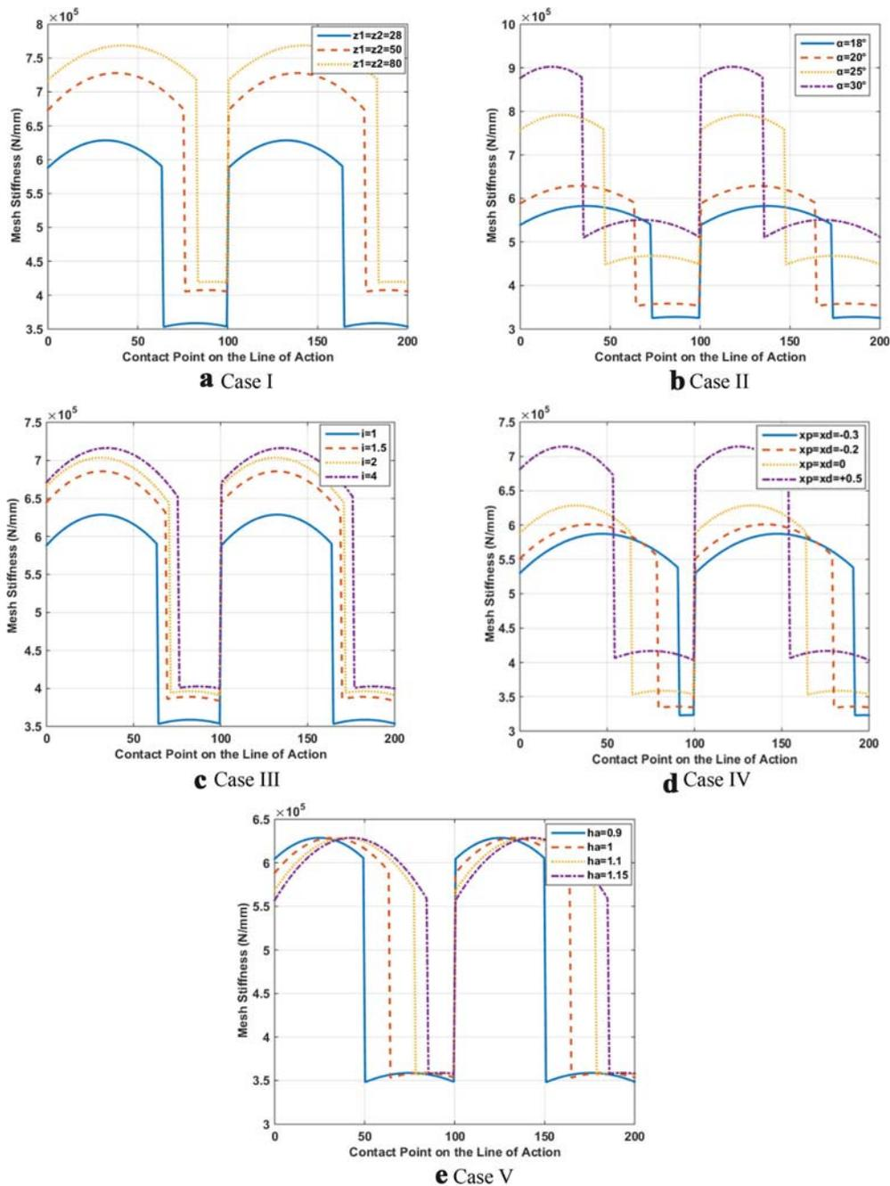
**Figure 7.** The effects of gear design parameters on mesh stiffness. a)  $z_1, z_2$ : Teeth number, b)  $\alpha$ : Pressure angle, c)  $i$ : Reduction ratio, d)  $x_p, x_d$ : Profile shifting factor, e)  $h_a$ : Addendum factor.
