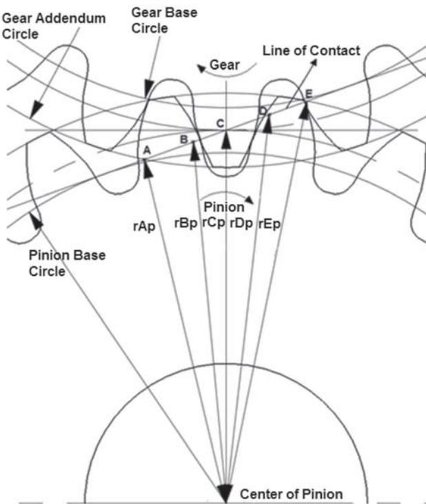
Figure 2. Meshing process in spur gear.
