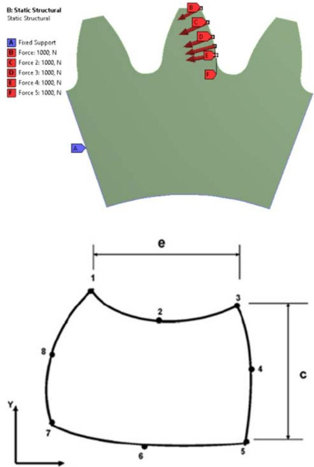
**Figure 1.** FEA boundary conditions and Plane-82 element model.
