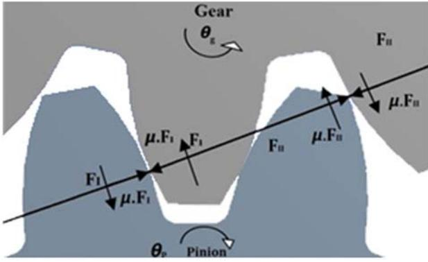
**Figure 5.** Schematic free body diagram of teeth pairs.
