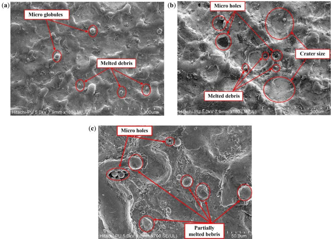
**Figure 4.** FESEM micrographs for the surface topography analysis of machined surface: (a) Experiment No. 2, (b) Experiment No. 9 and (c) Experiment No. 5.
