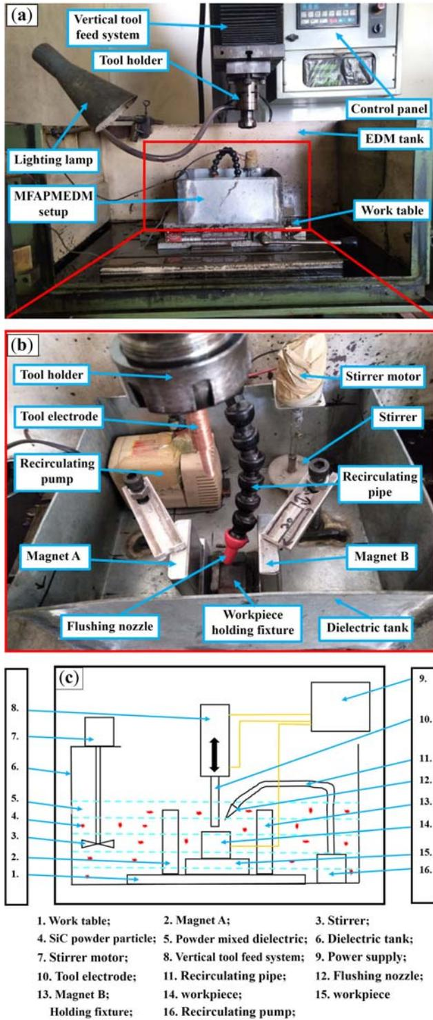
**Figure 1.** (a) ELEKTRAPULS CNC EDM machine, (b) apparatus for MFAPMEDM set-up and (c) schematic for the set-up.
