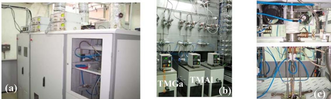
**Figure 2.** Real photographs of (a) indigenously developed nitride MOVPE system, (b) gas mixing system, and (c) MOVPE reactor.
