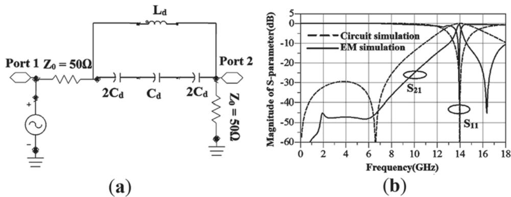
Figure 7. (a) Equivalent circuit model of DGS unit, (b) comparison between circuit and EM simulation.
