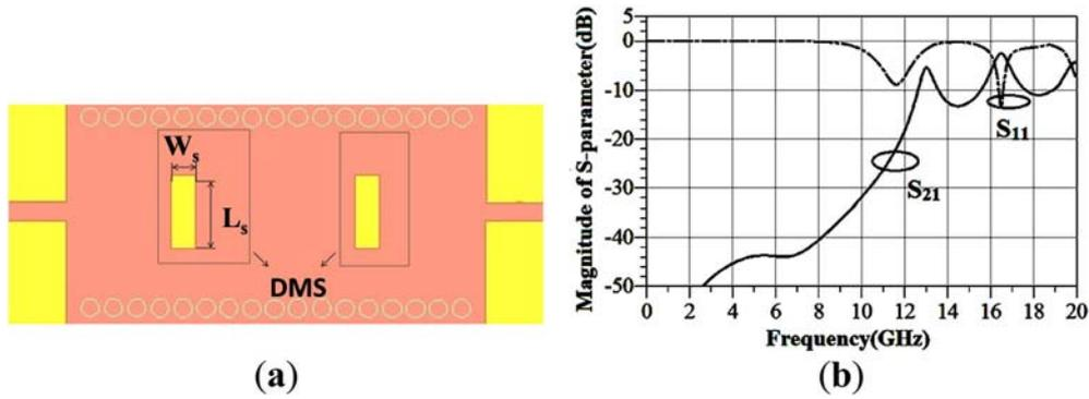
**Figure 3.** (a) Layout of the proposed SIW BPF with DMS, (b) simulated S-parameter of filter with DMS. The slot dimensions are  $W_s = 1.08$  mm,  $L_s = 3.2$  mm.
