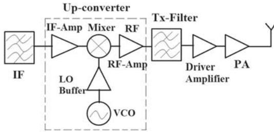
**Figure 1.** Ku-band transceiver up-converter block.
