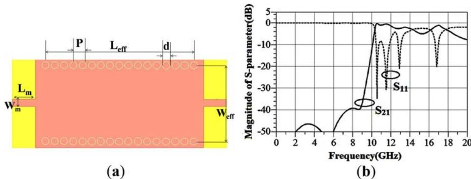
**Figure 2.** (a) Structure of SIW filter (without DMS and DGS), (b) simulated S-parameter of the SIW filter. The filter dimensions are  $L_{eff} = 16.5$  mm,  $W_{eff} = 8.6$  mm,  $L_m = 2.5$  mm,  $W = 0.8$  mm,  $P = 1$  mm,  $d = 0.82$  mm.
