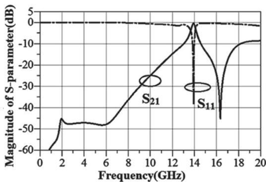
**Figure 5.** Simulated S-parameter of the proposed SIW BPF.
