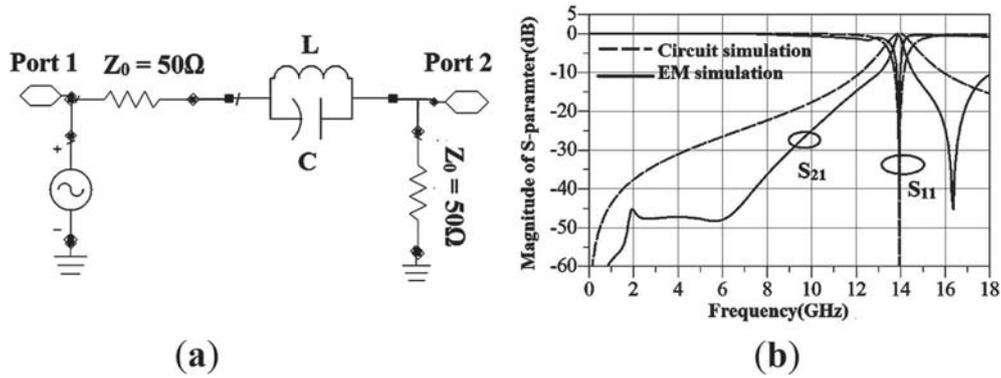
Figure 6. (a) Equivalent circuit model of DMS unit, (b) comparative results.
