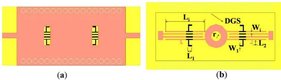
**Figure 4.** Layout of the proposed SIW BPF (with DMS and DGS). (a) top view, (b) bottom view.
