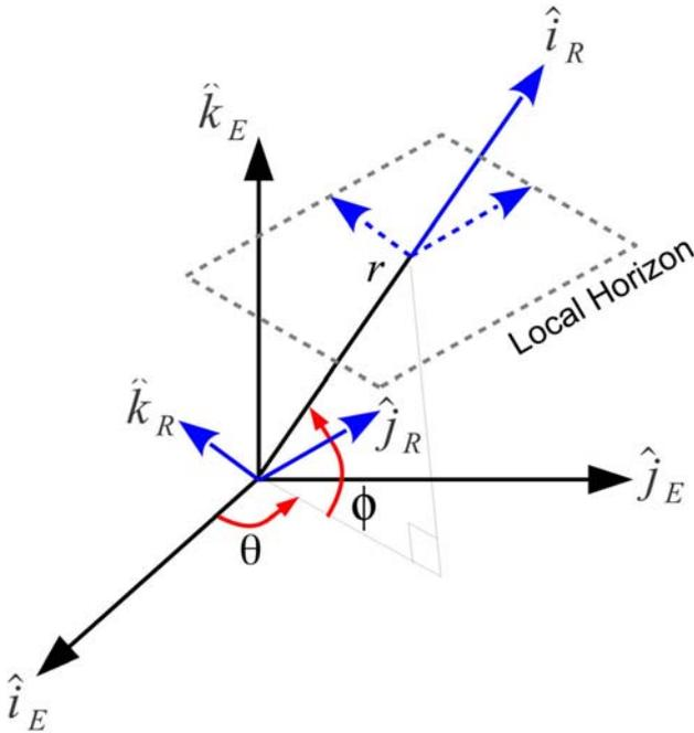
**Figure 4.** Radius Aligned Reference Frame (RARF)
