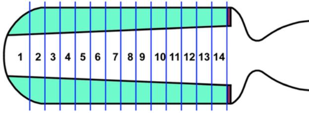
**Figure 3.** Schematic of a rocket motor with its grain divided into small elements.
