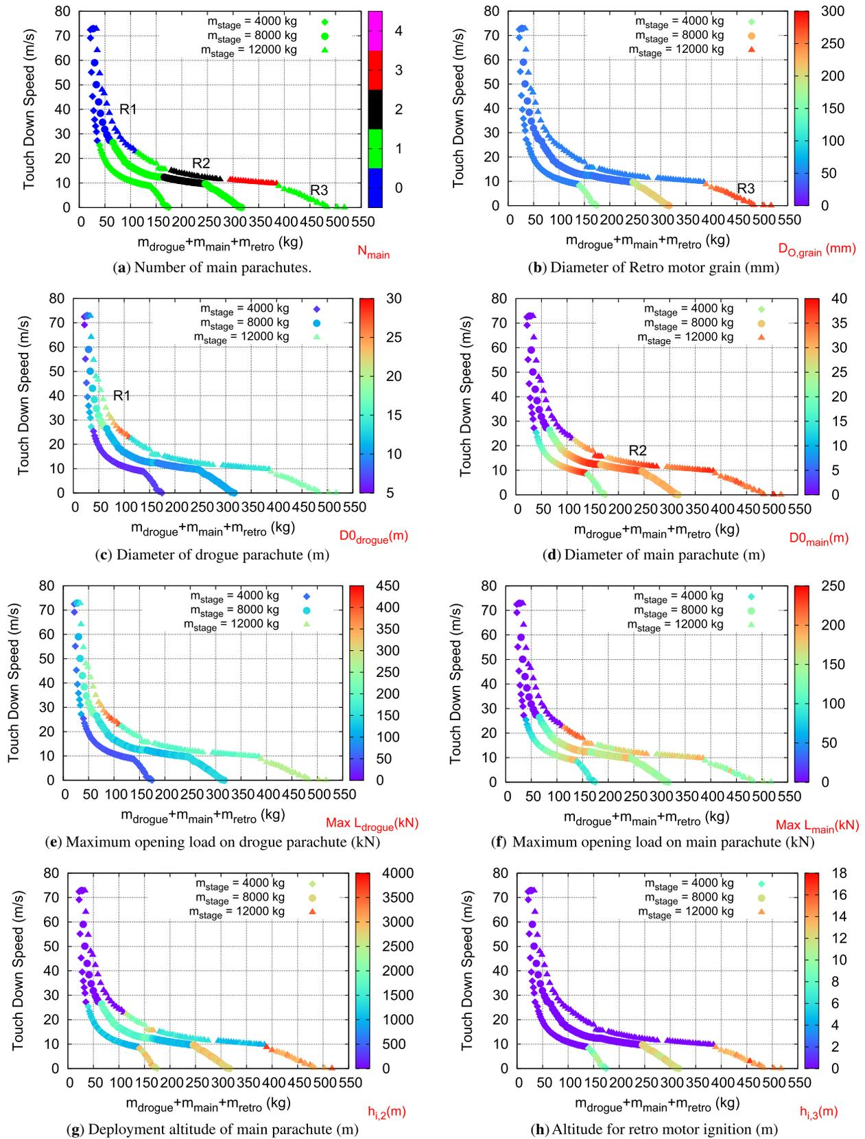
**Figure 6.** Results of deceleration system  $M^2DO$  for recovery of 4000, 8000 and 12000 kg stages.
