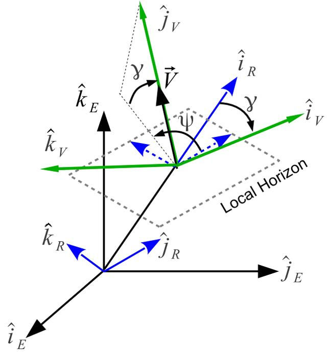
**Figure 5.** Velocity Aligned Reference Frame (VARF)
