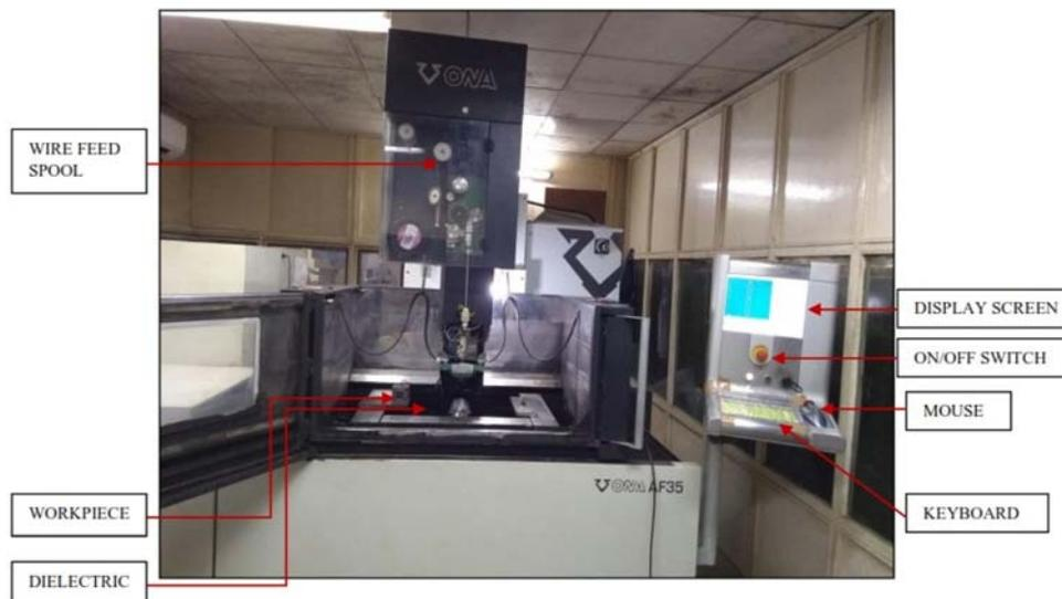
Figure 3. Experimental set-up of WEDM.
