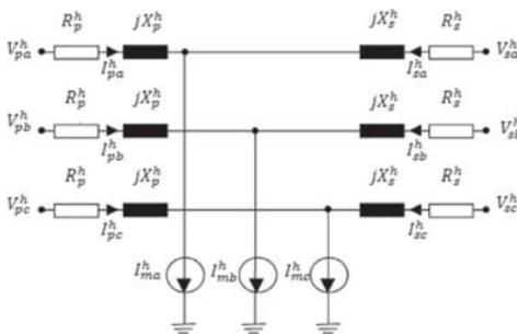
Figure 1. Harmonic field electrical circuit model of a power transformer.
