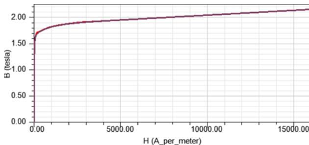
**Figure 3.** B-H curve for transformer core material.
