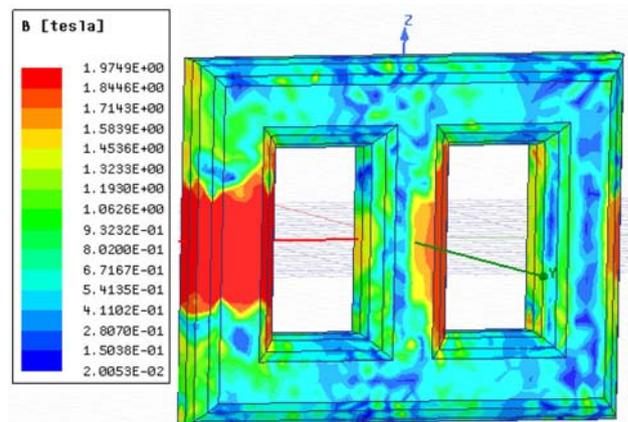
**Figure 5.** Flux distribution of transformer under harmonic.
