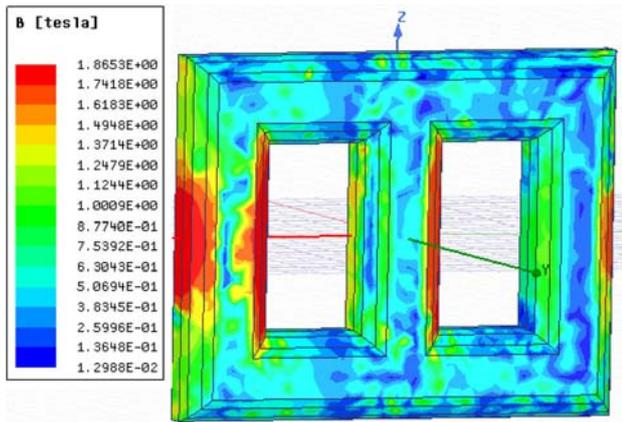
**Figure 6.** The flux distribution of the transformer under normal conditions.
