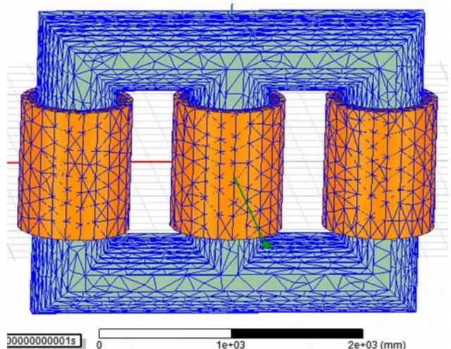
Figure 2. Transformer mesh model.
