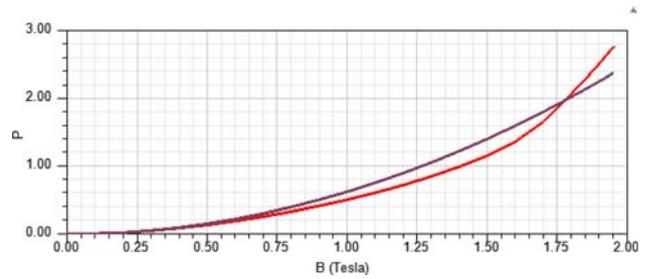
**Figure 4.** B-P curve for transformer core material.
