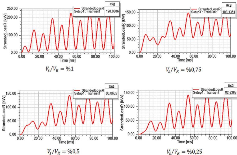
**Figure 7.** Loss curves of the transformer for harmonics.
