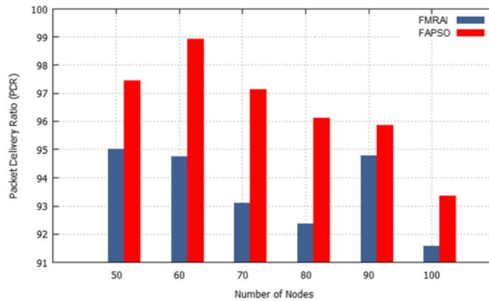
**Figure 4.** Nodes vs packet delivery ratio.
