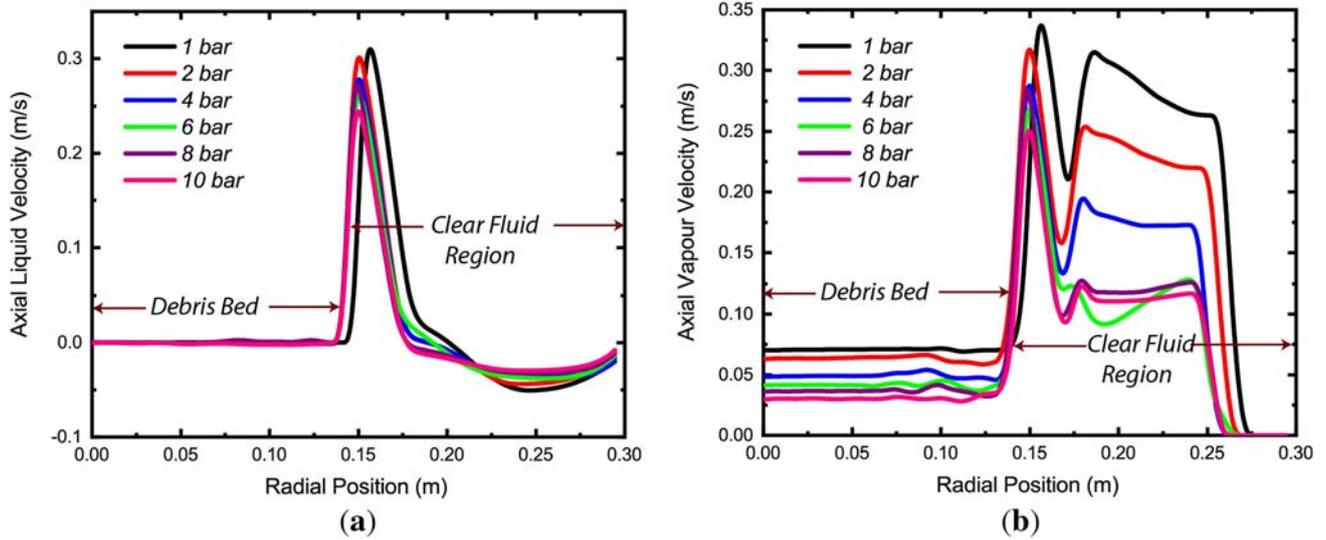
**Figure 8.** Axial velocity profiles of (a) liquid and (b) vapour at dryout conditions along the radial direction at  $z = 0.1$  for different pressures, considering saturated liquid.
