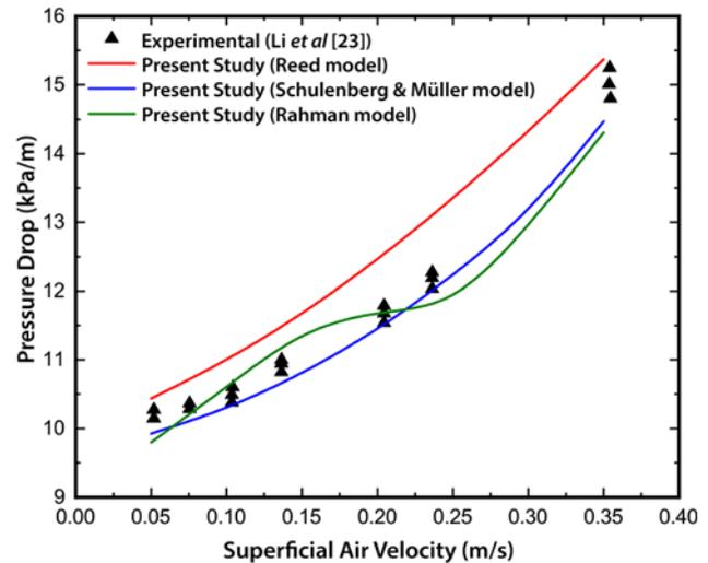
**Figure 3.** Comparison of pressure drop predicted by different drag models to experimental data of Li *et al* [23].
