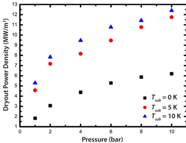
**Figure 5.** Variation in dryout power density with change in system pressure at three different subcooled conditions of flooding water.
