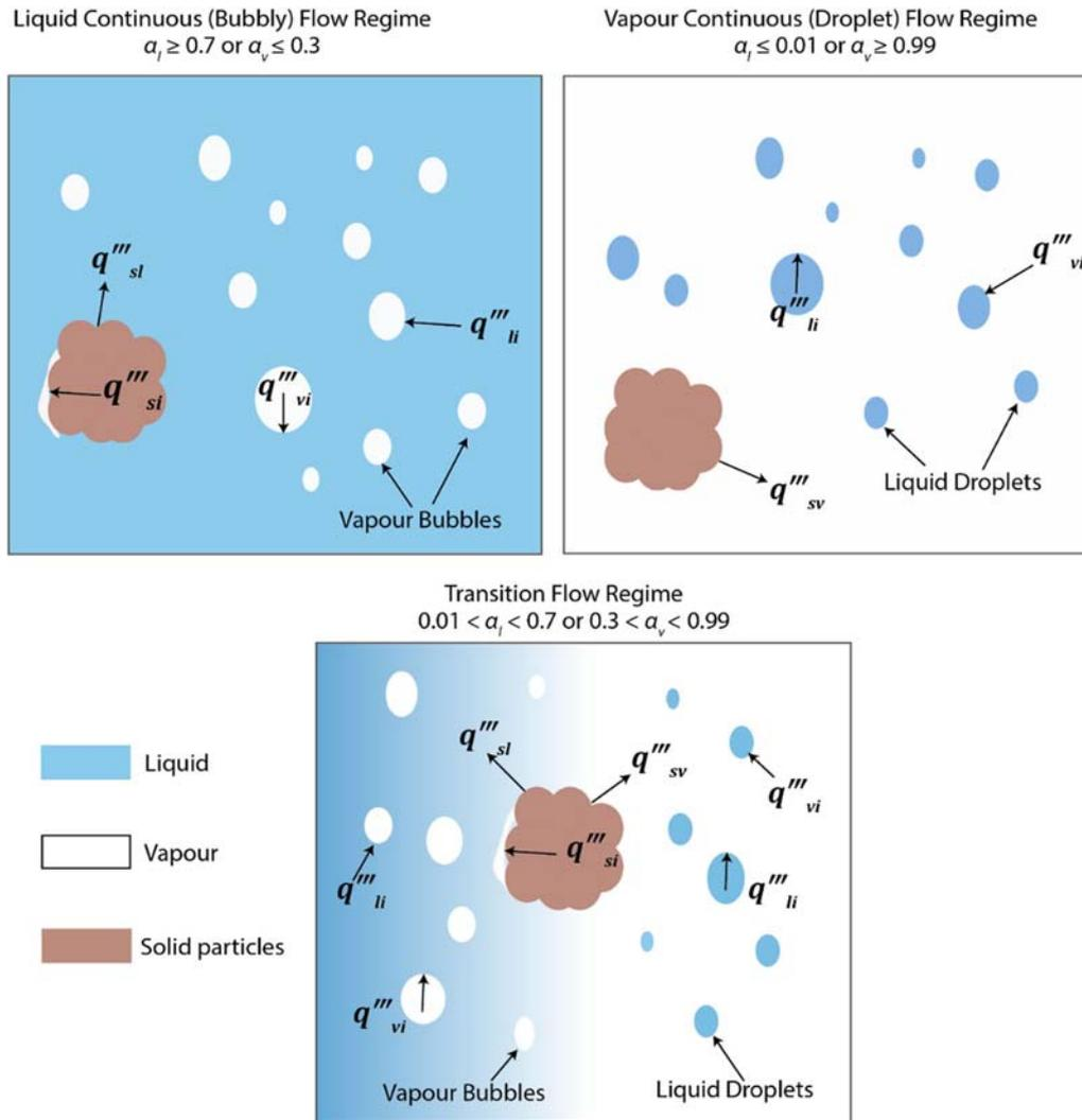
**Figure 2.** Heat transfer mechanisms considered among the heat-generating solid particles, liquid and vapour for different fluid flow regimes.
