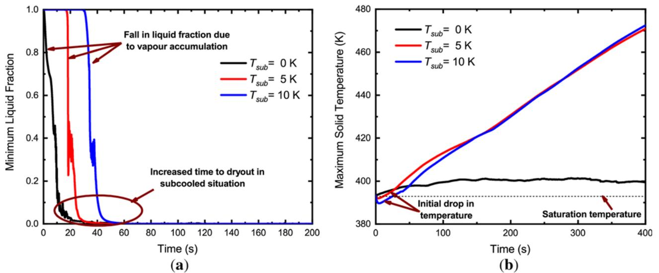
**Figure 9.** Temporal variation of (a) minimum liquid fraction and (b) maximum solid temperature at dryout conditions for different liquid subcoolings.
