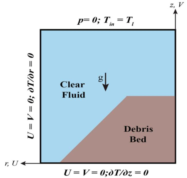
**Figure 1.** Schematic diagram of flow geometry and boundary conditions.
