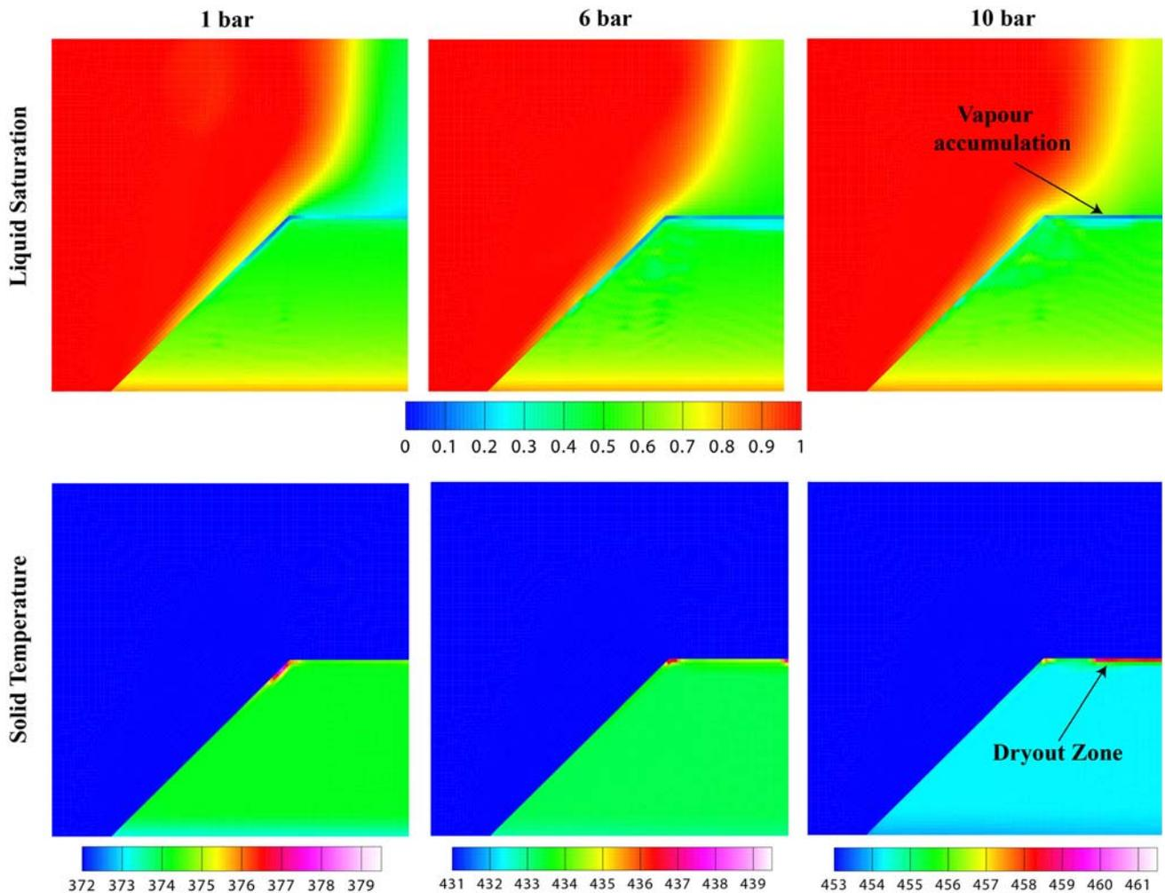
**Figure 7.** Liquid saturation and solid temperature distributions within the domain in a dryout situation at different system pressures, considering saturated conditions ( $T_{sub} = 0 \text{ K}$ ): 1 bar (200 s), 6 bar (200 s) and 10 bar (240 s).
