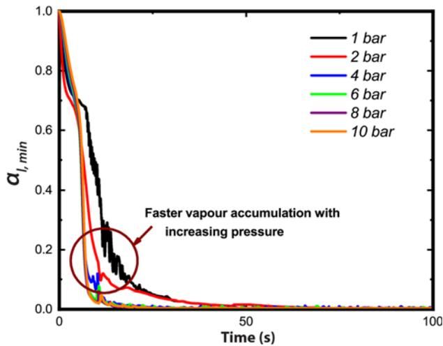
**Figure 6.** Temporal change in minimum liquid fraction at dryout condition for different system pressures, considering saturated liquid.
