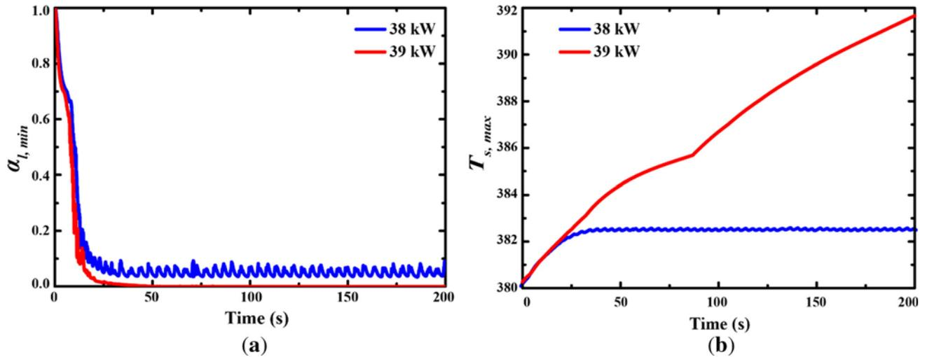
**Figure 4.** Temporal change of (a)  $\alpha_{l,min}$  and (b)  $T_{s,max}$  with Schulenberg and Muller drag model at two different heating powers.
