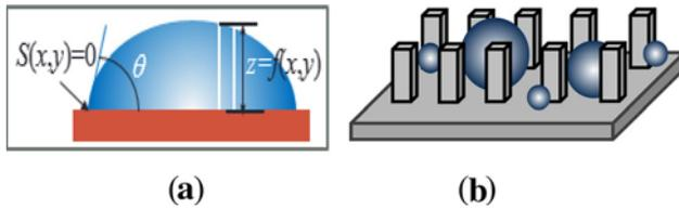
**Figure 1.** (a) A static sessile droplet on a smooth surface. (b) Picoliter-size droplets on a micropatterned surface.
