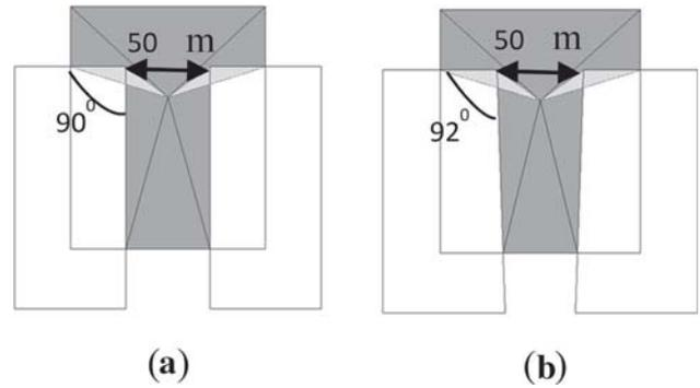
**Figure 9.** (a) parallel micro-pillars, (b)  $2^\circ$  tapered (non-parallel) micro-pillars.
