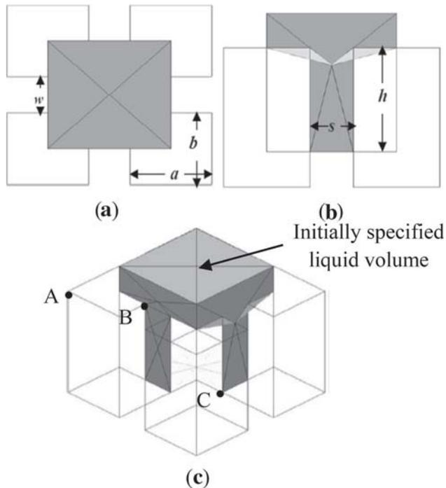
**Figure 2.** Geometry of the micropatterned surface (a) top view, (b) front view, (c) isometric view, showing the initial (assumed) shape of the dispensed liquid. Vertices A, B and C have different constraints as specified in section 3.2.
