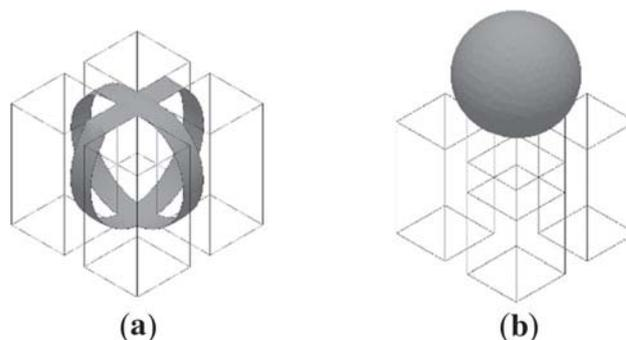
**Figure 5.** Droplet transitioning from the Wenzel state at  $0.65$  nL to Cassie-Baxter state after growing to  $1$  nL on the same surface having  $s = w = 30 \mu\text{m}$ , and  $\theta = 110^\circ$ .
