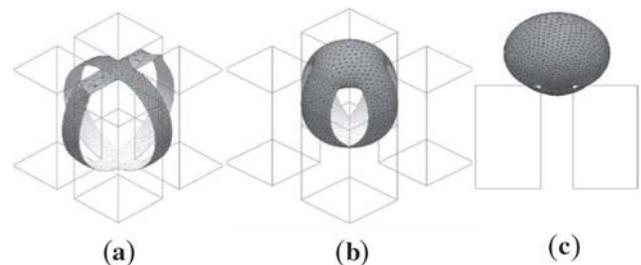
**Figure 3.** (a) Final equilibrium position in Wenzel state for a  $0.65 \text{ nL}$  water droplet when  $\theta = 100^\circ$  and  $s = w = 25 \mu\text{m}$ . For  $\theta = 135^\circ$  and  $s = w = 33 \mu\text{m}$  the droplet rises upward (b), and eventually assumes a stable Cassie state (c).
