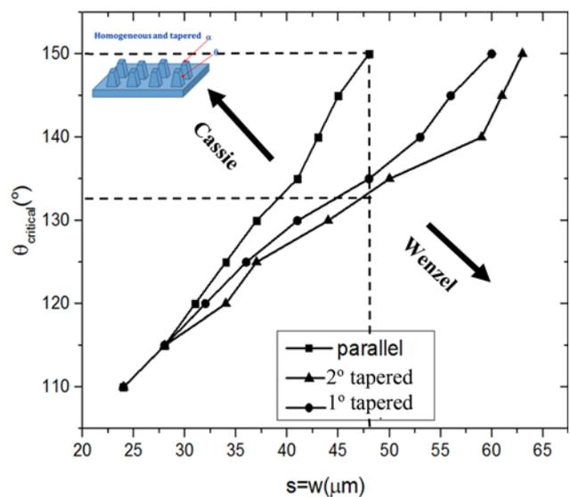
**Figure 10.** Variation of  $\theta_{critical}$  as a function of micro-pillar spacing for three different micro-pillar structures for a droplet volume of 0.65 nL.
