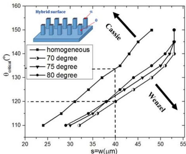
**Figure 6.** Variation of  $\theta_{critical}$ , for a 0.65 nL droplet, as a function of micro-pillar spacing ( $s = w$ ) for three different values of  $\alpha$  ( $70^\circ$ ,  $75^\circ$  and  $80^\circ$ ).
