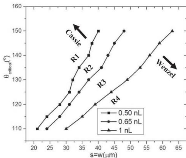
**Figure 4.** Variation of  $\theta_{critical}$  as a function of micro-pillar spacing for three different droplet volumes. Regime R1 denotes Cassie-Baxter state for all droplets, R4 denotes Wenzel state for all, while R2 and R3 denote Cassie-Baxter for the larger and Wenzel state for the smaller droplets.
