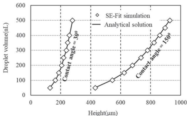
**Figure 12.** Droplet volume versus maximum droplet height for sessile droplets on smooth surfaces for two different sessile-droplet contact angles. Data points show SE-Fit simulation results, line denotes analytical solution following spherical cap assumption [19].
