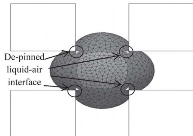
**Figure 7.** De-pinning of droplet having volume of 0.65 nL, side wall contact angle  $\theta = 145^\circ$ , pillar-top contact angle  $\alpha = 70^\circ$  and  $s = w = 53 \mu\text{m}$ .
