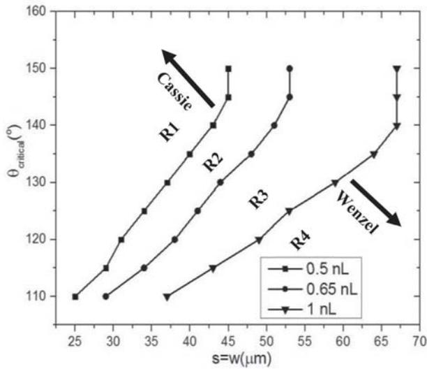
**Figure 8.** Variation of  $\theta_{critical}$  as a function of micro-pillar spacing for three different droplet volumes. The pillar top contact angle  $\alpha = 80^\circ$  for all cases. Regimes R1 through R4 denote the Cassie or Wenzel behaviors of sessile droplet as explained in figure 4.
