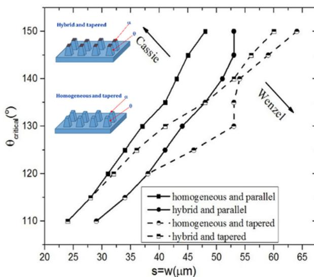
**Figure 11.** Variation of  $\theta_{critical}$  as a function of micro-pillar spacing for different micro-pillar structures for a droplet volume of 0.65 nL.
