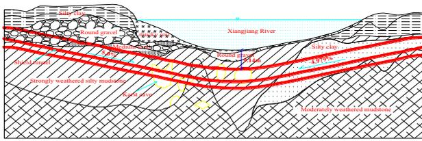
Figure 7. Geological section of the Hejiangtao Tunnel.
