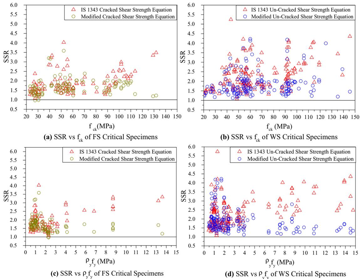
**Figure 7.** Variation of Shear Strength Ratio with Parametric Values.
