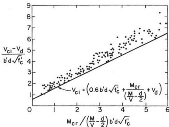
**Figure 2.** Experimental Data for Calibration of ACI 318-63 Flexure-Shear Strength.
