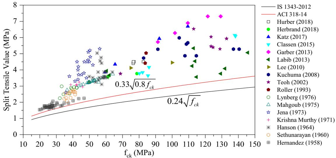
Figure 3. Variation of Split Tensile Strengths with Cube Strength of Concrete.
