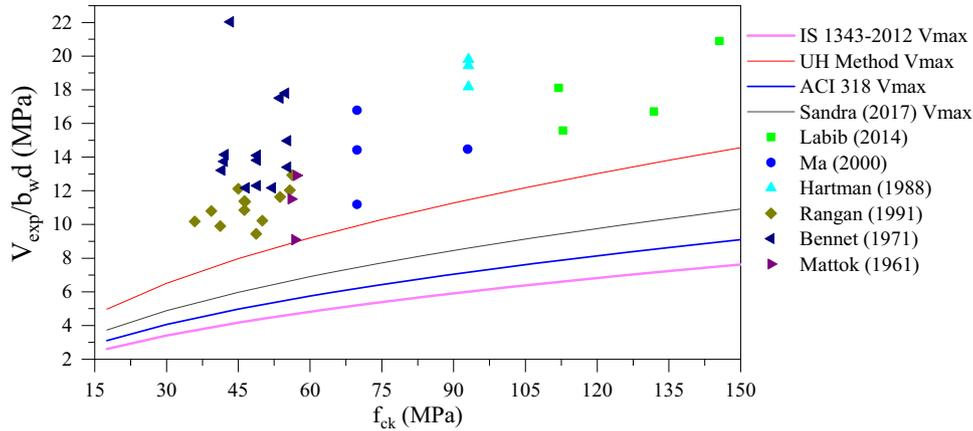
Figure 5. Variation of Maximum Shear Strength with Concrete Strengths.
