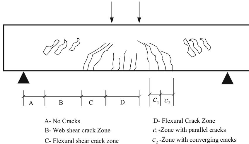
**Figure 1.** Description of Crack Zones in PC Member.
