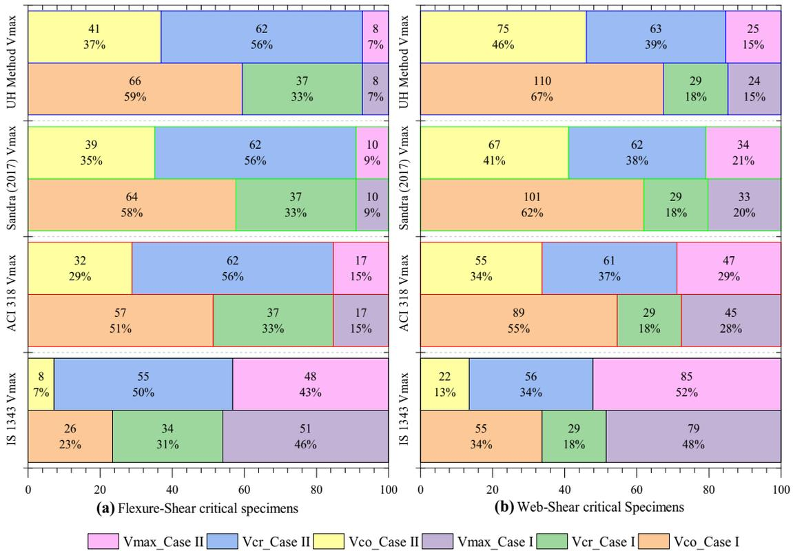
Figure 6. Governing Failure Mode Comparison of Flexure-Shear and Web-Shear Critical Specimens.
