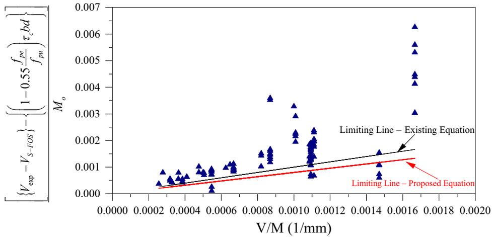
Figure 4. Variation of Cracked Shear Strength with V/M.
