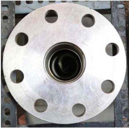
**Figure 3.** Photograph of heater-housing assembly.
