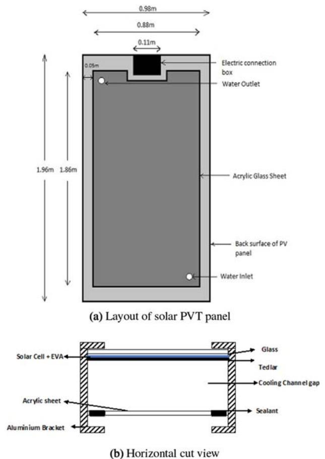
**Figure 1.** Schematic of PVT panel.
