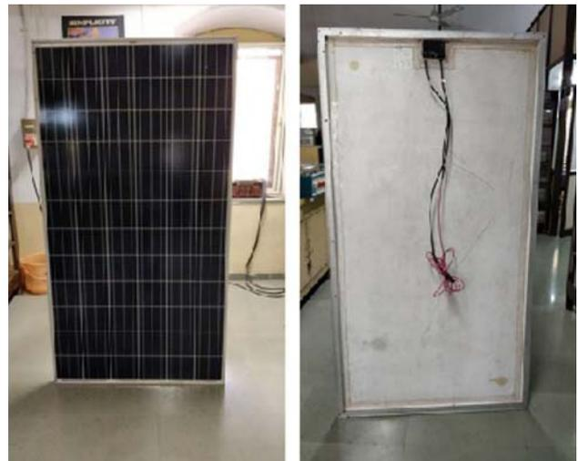
**Figure 2.** Front and back view of the proposed PVT panel.
