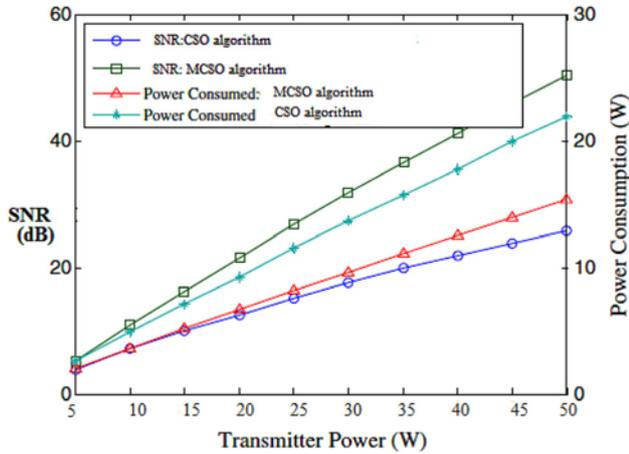
**Figure 2.** SNR and power consumption as a function of transmitted power. The variation of SNR and power consumption at selected relay(s) is analysed for CSO and MCSO algorithms for different values of input transmission power from 5 to 50 W.
