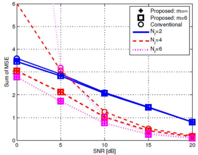
**Figure 7.** Performance comparison in terms of sum of MSE as a function of SNR. Here analysis is done for 3 different number of relays selected using MCSO algorithm. Each case of  $N_r = 2, 4$  and  $6$  is compared for 3 distinct aspects of JBF—conventional, proposed for  $m = \infty$  and proposed for  $m = \hat{m}$  cases.
