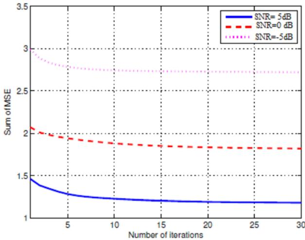
**Figure 5.** Convergence comparison. Convergence rate of proposed JBF with time optimization ( $m = \hat{m}$  case) is depicted for distinct SNR regimes  $-5, 0$  and  $5$  dB.
