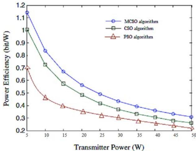
**Figure 3.** Performance comparison in terms of power efficiency as a function of transmitter power. The power efficiency at selected relay(s) is analysed by varying input transmitter power from 5 to 50 W and performance is compared for conventional PSO, CSO with proposed MCSO.
