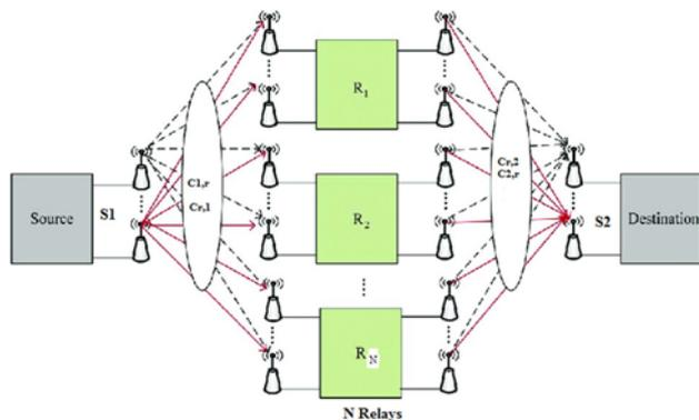
**Figure 1.** System model. Communication between two source nodes equipped with multiple antennas is facilitated by ‘ $N$ ’ relay nodes with multiple antennas. Channel State Information matrices are explicitly mentioned.
