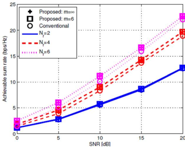
**Figure 6.** Performance comparison of JBF in terms of ASR as a function of SNR. Here analysis is done for three different numbers of relays selected using MCSO algorithm. Each case of  $N_r = 2, 4$  and  $6$  is compared for three distinct aspects of JBF—conventional, proposed for  $m = \infty$  and proposed for  $m = \hat{m}$  cases.
