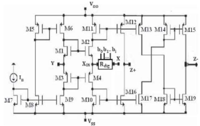
Figure 4. Resistance tunable dual output CCCII.
