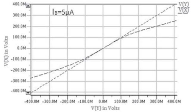
Figure 6. DC analysis for voltage transfer from terminal Y to X.
