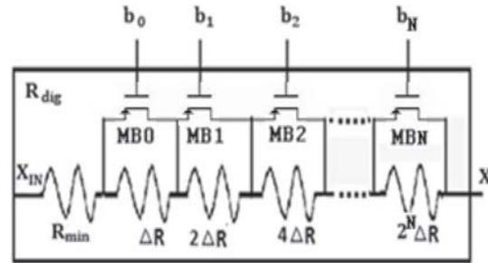
Figure 5. Externally driven digitally controlled resistor block.
