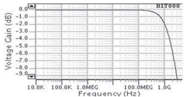
**Figure 10.** Frequency response for (a) voltage gain at X terminal.
