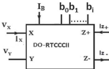
Figure 3. Block diagram of resistance tunable dual output CCCII.
