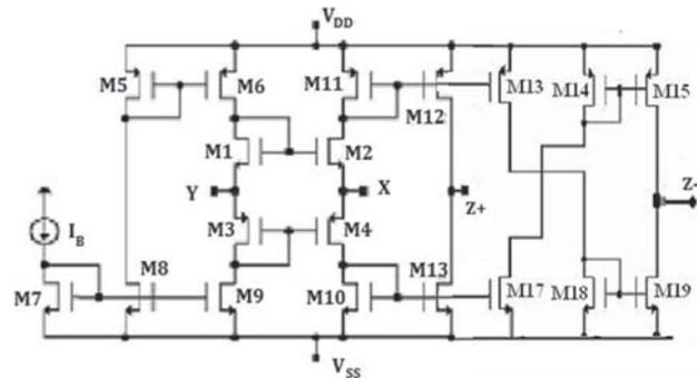
Figure 2. CMOS based circuit of DO-CCCII.
