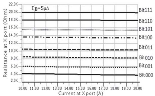
Figure 8. Resistance of X terminal versus (a) X terminal current.
