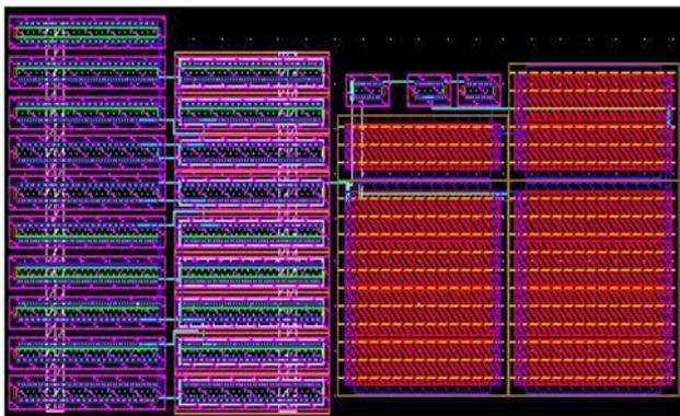
**Figure 12.** Layout view of proposed DO-RTCCCI.
