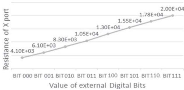
**Figure 9.** Resistance of X terminal versus different digital bits.
