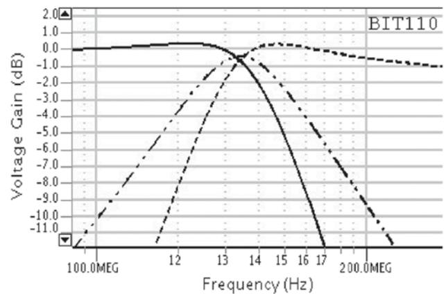
**Figure 14.** Frequency responses for low pass, high pass and band pass filters.
