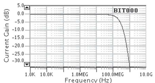
**Figure 11.** Frequency response for current gain at terminal Z.
