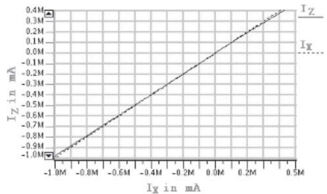
Figure 7. DC analysis for current transfer from terminal X to Z.
