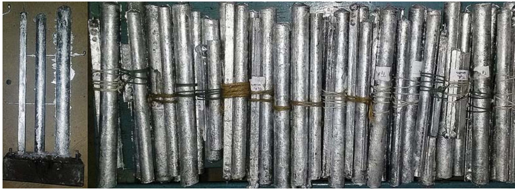
Figure 2. Fabricated samples Al6063/BR composite through advanced stir cast process.
