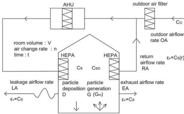
**Figure 2.** Basic cleanroom airflow configuration.
