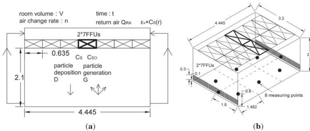
Figure 3. Cleanroom airflow configuration.
