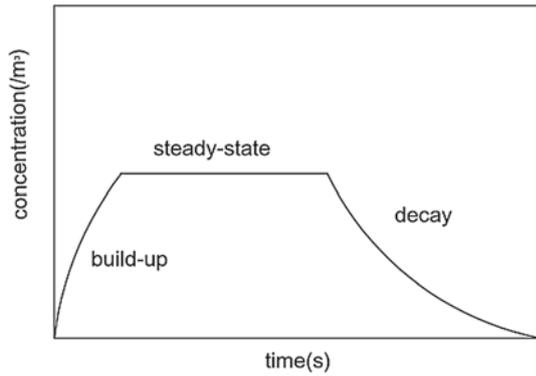
**Figure 1.** Build-up, steady state, and decay of airborne contamination in ventilated room.
