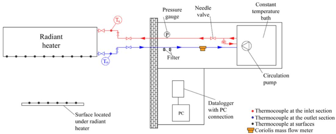
(a) Schematic of experimental set-up
