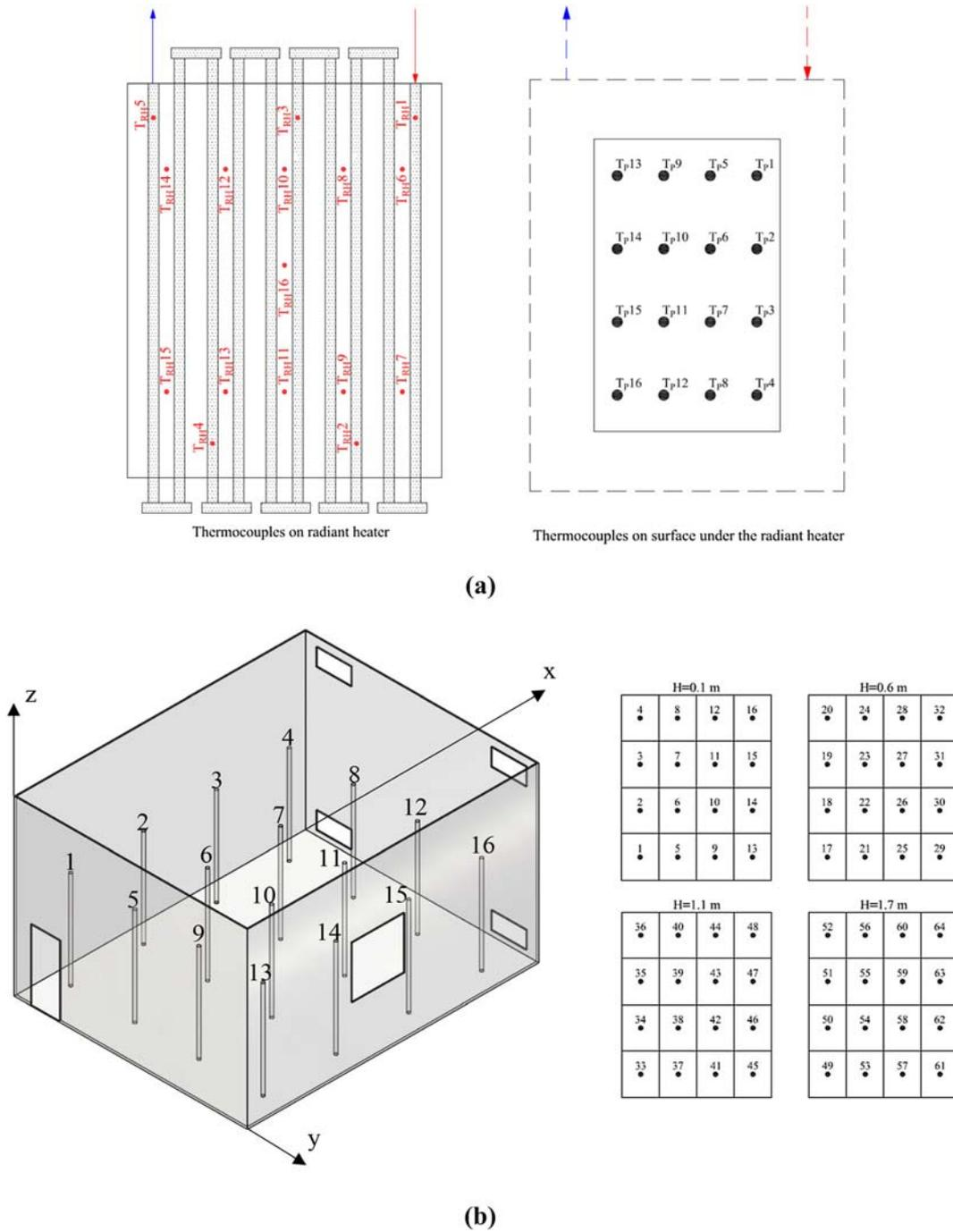
**Figure 2.** Temperature measurement locations. (a) measurement locations on panel and plate, (b) measurement locations inside the test room.
