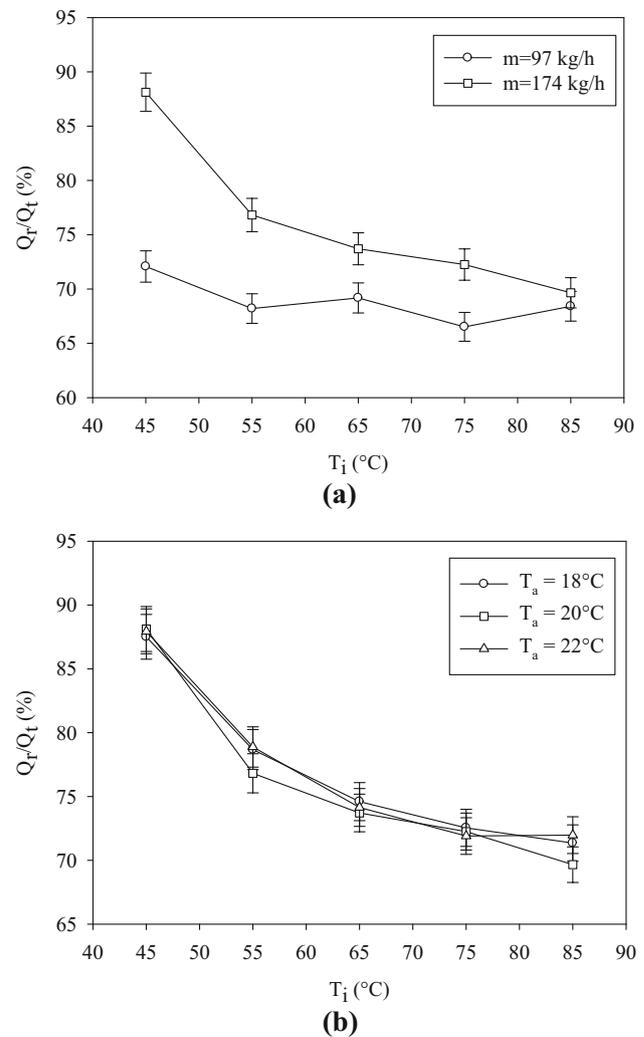
**Figure 5.** Fraction of heat transfer by radiation to the total heat output of the radiant panel (a) effect of mass flow rate ( $T_a = 20$  °C), (b) effect of room temperature ( $\dot{m} = 174$  kg/h) with change in the inlet temperature.
