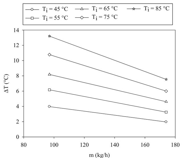
**Figure 4.** Change of temperature difference between inlet and outlet with mass flow rate for different inlet temperatures ( $T_a = 20^\circ\text{C}$ ).
