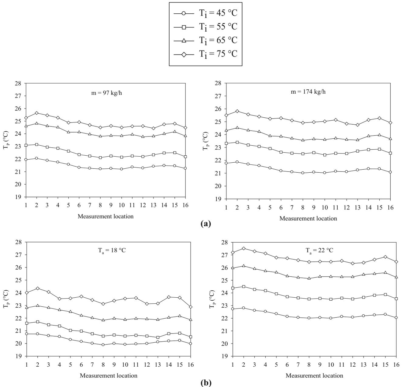
**Figure 8.** Local temperature distributions on the plate located below the radiant heater (a) effect of different mass flow rates ( $T_a = 20\text{ }^\circ\text{C}$ ), (b) effect of room temperature ( $\dot{m} = 174\text{ kg/h}$ ).
