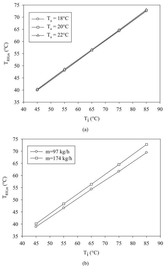
**Figure 6.** Effect of different operating conditions on radiant heater arithmetic mean surface temperature with changes in the inlet temperature (a) effect of room temperature ( $\dot{m} = 174$  kg/h), (b) effect of mass flow rate ( $T_a = 20$  °C).
