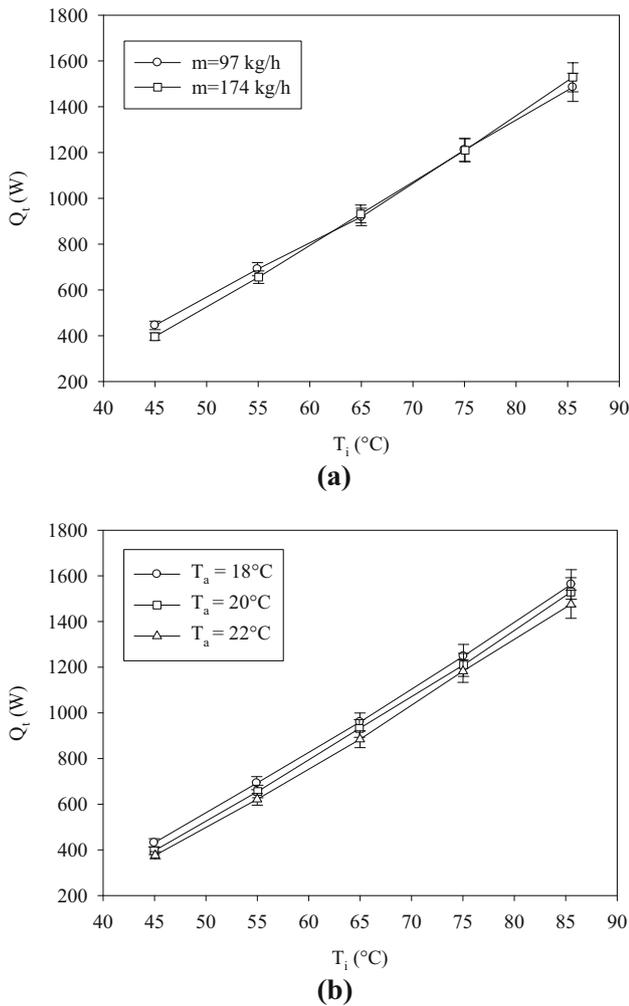
**Figure 3.** Heat output of hydronic radiant heater for different working conditions with changes in the inlet temperature (a) effect mass flow rate ( $T_a = 20^\circ\text{C}$ ), (b) effect of room temperature ( $\dot{m} = 174\text{ kg/h}$ ).
