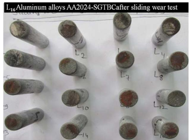
**Figure 2.** Worn surface of coated AA2024-T351 substrate.
