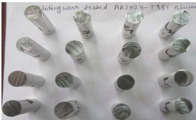
**Figure 1.** Worn surface of uncoated AA2024-T351 substrate.
