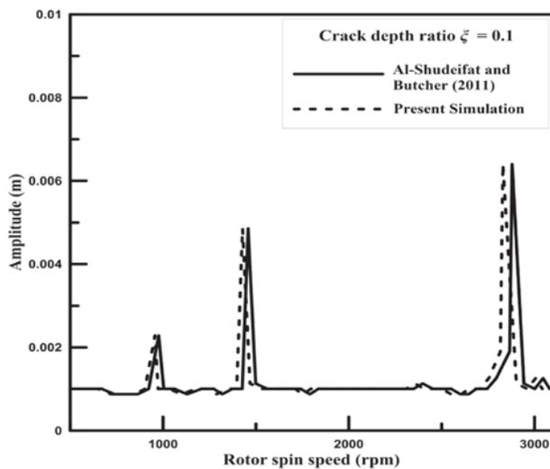
**Figure 4.** Unbalance response validation.
