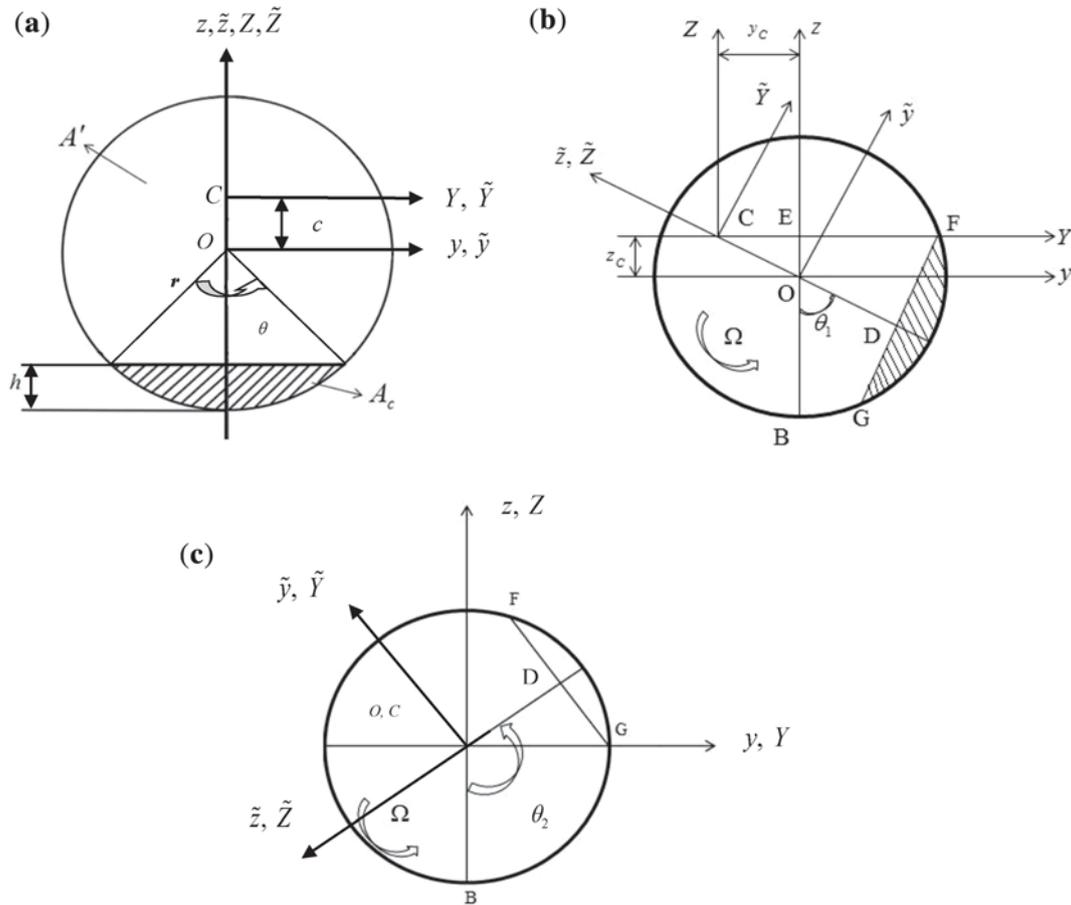
**Figure 1.** Different orientation of cracked element rotor cross-section a) At rest, b) When the crack starts to close and c) When the crack becomes full close.
