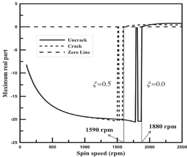
**Figure 6.** Decay rate plot, uncracked vs. cracked propeller shaft.
