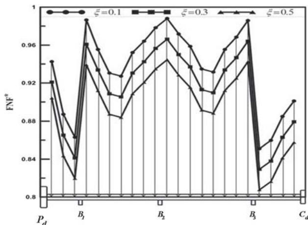
**Figure 11.** Non-dimensional first natural frequency vs. crack location for different crack depth ratio.
