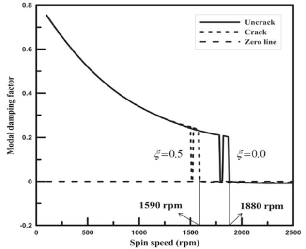
**Figure 8.** Modal damping factor, uncracked vs. cracked propeller shaft.
