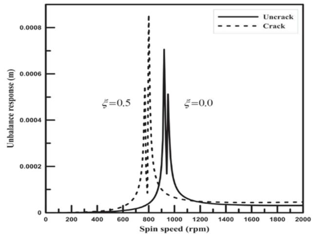
**Figure 9.** Mass unbalance response, uncracked vs. cracked propeller shaft.
