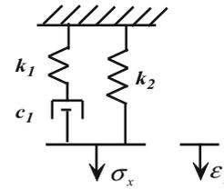
Figure 2. Standard 3- Element Model.
