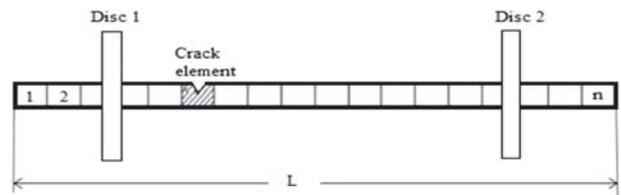
**Figure 3.** Discretized rotor disk system (Al-Shudeifat and Butcher [12]).
