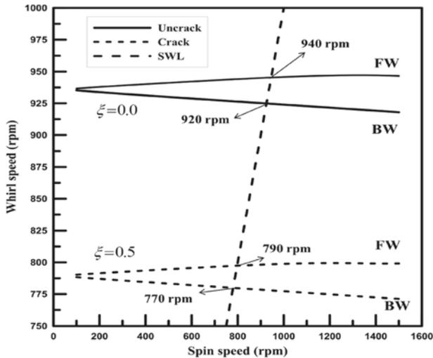
**Figure 7.** Campbell diagram, uncracked vs. cracked propeller shaft.
