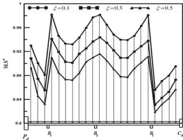
**Figure 10.** Non-dimensional stability limit of spin speed vs. crack location for different crack depth ratio.
